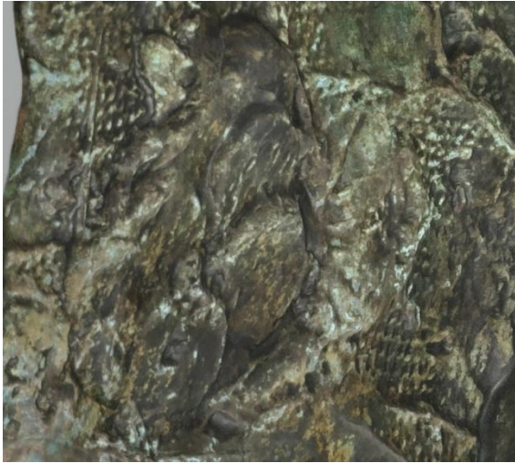
Fig. 3.2. Imprint of cloth still visible on the surface of the finished bronze. Detail of the base of the Laren Thinker .
