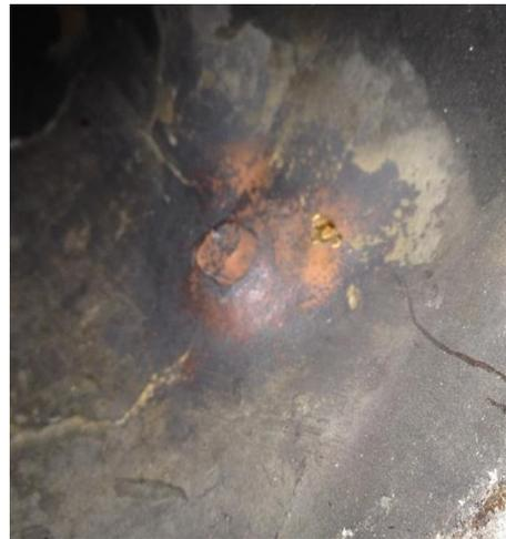
Fig. 5.59. A brazed plug inside the Yale *Thinker*, note the heat discoloration.
