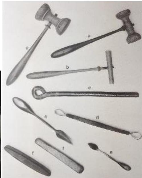
Fig. 4.26. Various sand moulding tools. (from Baudry 2005, 282)
