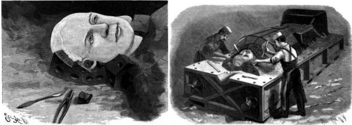
Fig. 4.27. The moulding, in 1890, of John Quincy Adams Ward's statue of Henry Ward Beecher in a sand piece mould (with more than a thousand false cores) by the Henry-Bonnard Bronze Company of NYC. Notice the concave keys in the surface of the false-cores on the left image. (images from Anonymous. 1891. 'Casting the Henry Ward Beecher Statue for the City of Brooklyn'. *Scientific American*, Vol. LXIV.-No. 26, June 27)
