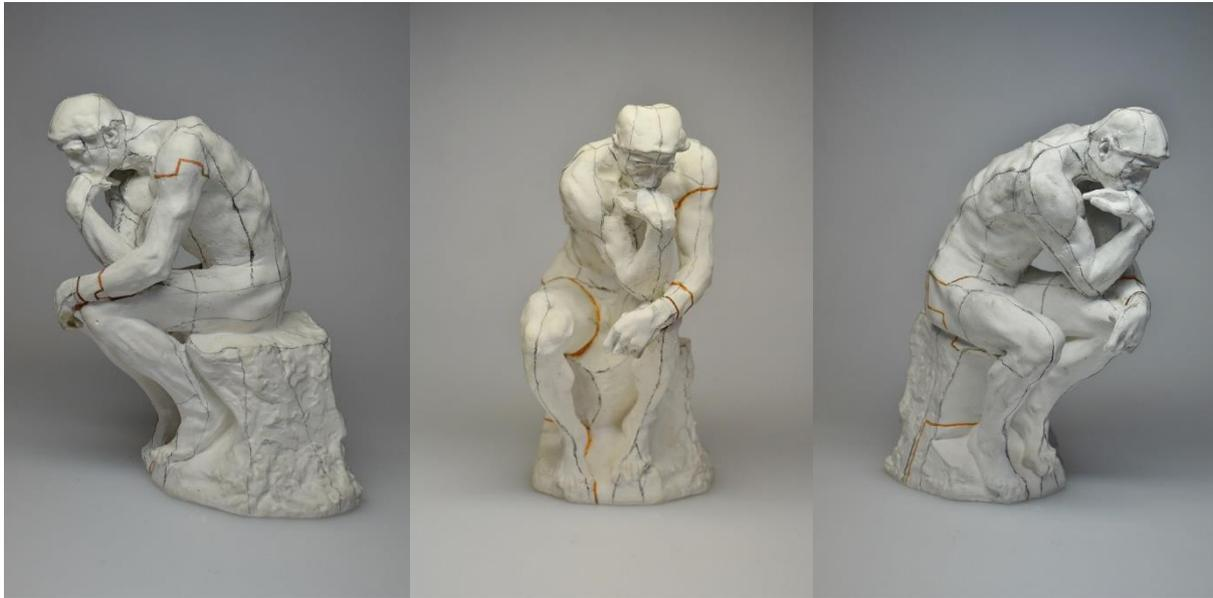
Fig. 4.23. Three different views of the same reduced plaster model of the *Thinker*, the lines on the surface indicate the cutting lines of the false cores, as observed on the original plaster foundry model (S.2840). The orange lines are where the original foundry plaster is divided in separate parts.
