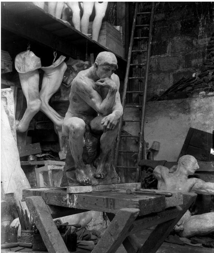
Fig. 4.66. The original sized *Thinker* in the Rudier Foundry during the chasing process. The chasing hammer can be seen lying on the working platform, with underneath in the left corner the chasing punches visible. Image taken probably between 1920 and 1940.<sup>711</sup> (image <http://mymagicalattic.blogspot.nl/2014/09/mapplethorpe-rodin-at-musee-rodin-paris.html>.> [accessed 22 June 2018])
