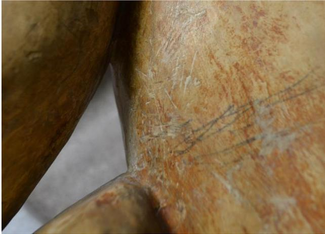
Fig. 4.16. A detail of the underside of the left thigh of foundry plaster S.3189 showing pencil marks from the moulding.
