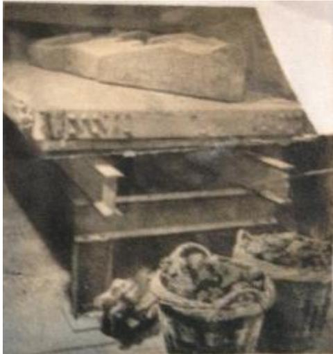
Fig. 4.47. Mould-pieces in the drying oven of the Rudier foundry. (between 1934-52) (image from an undated Dutch article called “*Hoe men bronzen beelden giet*” in the Malvina Hoffman papers, Box 15.2, Special Collections Getty Research Institute, Los Angeles.)
