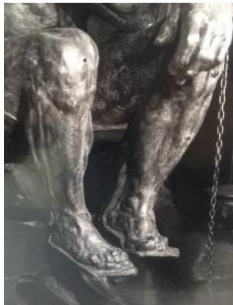
Fig. 4.56. Detail of the monumental *Thinker* during finishing, with the holes still visible where the core support irons have been removed. Image taken by Robert Doisneau in the Alexis Rudier foundry at Malakoff in Paris in 1950. (image Doisneau estate)
