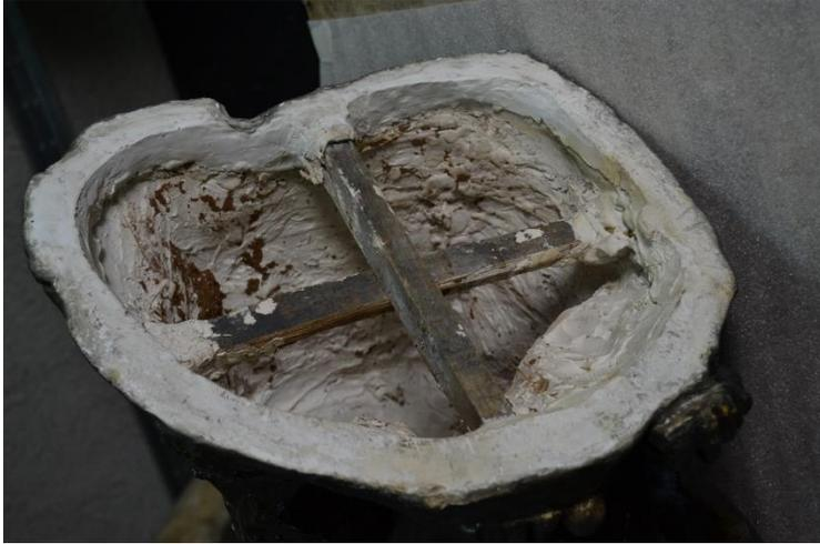
Fig. 4.12. Underside of the base of foundry plaster S.2520, with the wooden reinforcement visible.
