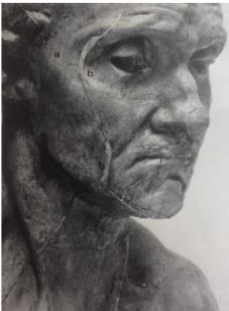
Fig. 4.55. Unfinished face of Rodin's *Jean d'Aire*, a sand mould cast by the Godard foundry of Paris in 1973. The remnants of runners (b) are still visible as are flashing fins from the false-cores (a) which have not been removed. (from Arminjon 1998, 83)
