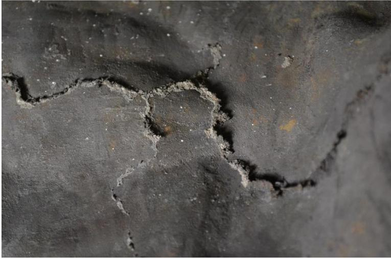
Fig. 4.42. A detail of the veining visible on the interior surface of the Brussels Petermann *Thinker*.
