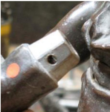
Fig. 4.4. Detail of a pattern at the Chardon & Petit Fils foundry in Paris, illustrating the male part of a sleeve or Roman joint. (image Jane Bassett, Getty Conservation Institute, Los Angeles)
