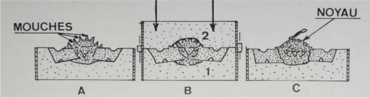
Fig. 4.36. Drawing illustrating the steps in making a sand core with the aid of flies, the so-called *mouchetage*. When the cope (2) is lowered down onto the drag, the flies are compressed (B). This determines the outline of the top half of the mould and the spaces between the flies can now be filled with moulding sand to complete the outline of the core (C). (from Rama 1988, 166)
