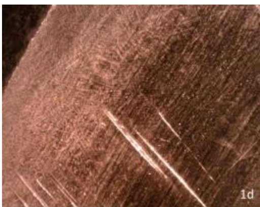
Fig. 1d in-situ metallography of the cutting surface after etching with FeCl 3 + HCl + EtOH. The highest magnification possible with the Dyna lite was x 90 and was sufficient to clearly distinguish the presence of dendrites on the etched surface, but not enough to investigate other morphological features.
