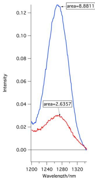
NIR emission spectra displaying singlet oxygen emission generated by ZnPC in DMF (blue) and by acetylated lignin (OL) in DMF (red) obtained from samples with matched absorption of 0.1 at 350 nm. The area under the red spectrum is ca. 30% of that of the blue spectrum. A 850 nm cutoff filter was used in the emission channel.
