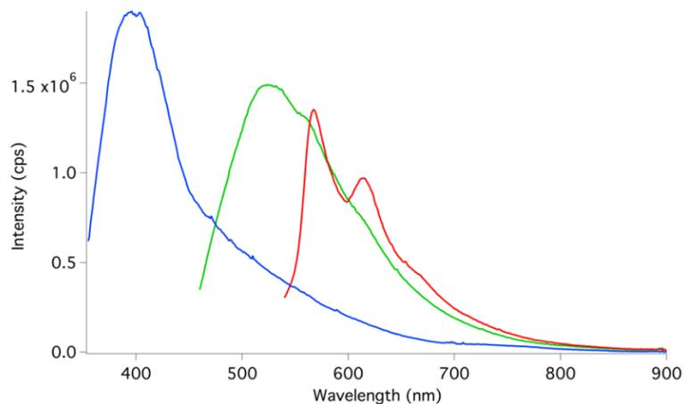
Front face emission spectra of acetylated lignin (OL) in DMF using 350 nm (blue), 450 nm (green) and 525 nm (red) excitation. Slits were 1, 2 and 3 nm respectively for excitation path. Slit was 5 nm for emission path for all. Second order effects were suppressed with cut-off filters.
