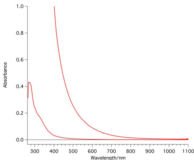
UV-Vis absorption spectra of two DMF solutions of acetylated lignin (OL). A maximum at 271 nm, a shoulder at 332 (diluted sample) and an absorption onset around 900 nm can be observed (high concentration).
