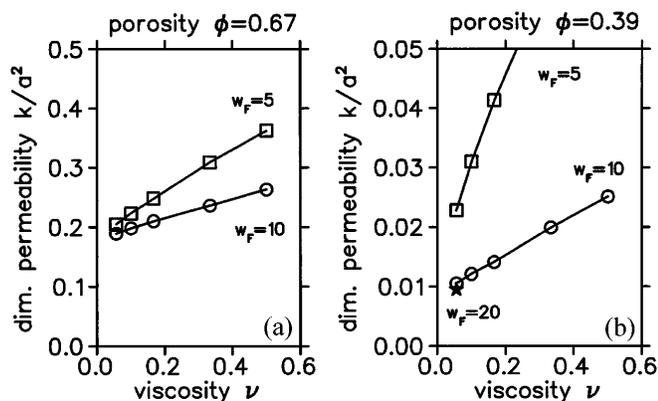
FIG. 3. Calculated dimensionless permeability  $k/a^2$  as a function of viscosity  $\nu$  for two test samples with porosities (a)  $\phi = 0.67$  and (b)  $\phi = 0.39$ . Here  $a = w_F/2$  is the hydraulic radius of the fibers. The fiber widths (grid resolutions) are  $w_F = 5$  (squares), 10 (circles), and 20 (star).
