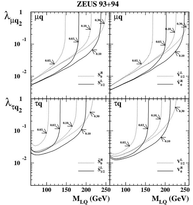
**Fig. 8.** The upper limit on the coupling at the decay vertex ( $\lambda_{\ell q_2}$ ) vs. leptoquark mass  $M_{LQ}$ , for several values of the first-generation coupling at the production vertex ( $\lambda_{eq_1}$ ). Each curve is labeled by the value of  $\lambda_{eq_1}$ . The dotted curves are for  $F = 2$  leptoquarks and the solid curves are for  $F = 0$  leptoquarks
