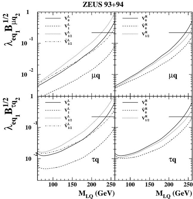
**Fig. 6.** The upper limit on the coupling at the production vertex ( $\lambda_{eq_1}$ ) times the square root of the branching fraction to the  $\mu q$  or  $\tau q$  final state ( $B_{\ell q_2}$ ) vs. leptoquark mass  $M_{LQ}$ , at 95% CL for vector leptoquarks. The horizontal line indicates nominal electromagnetic coupling ( $\lambda_{e q_1}^2 = 4\pi\alpha = 4\pi/128$ ) and  $B_{\ell q_2} = 0.5$
