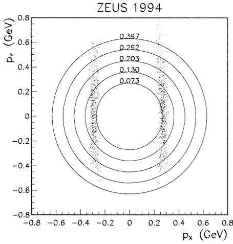
**Fig. 8.** Scatter plot of the  $X$  and  $Y$  components of the scattered proton momentum as measured by the LPS for the accepted events. The continuous curves correspond to the indicated values of  $|t|$  (in  $\text{GeV}^2$ ), which were used as limits of the bins in Fig. 13
