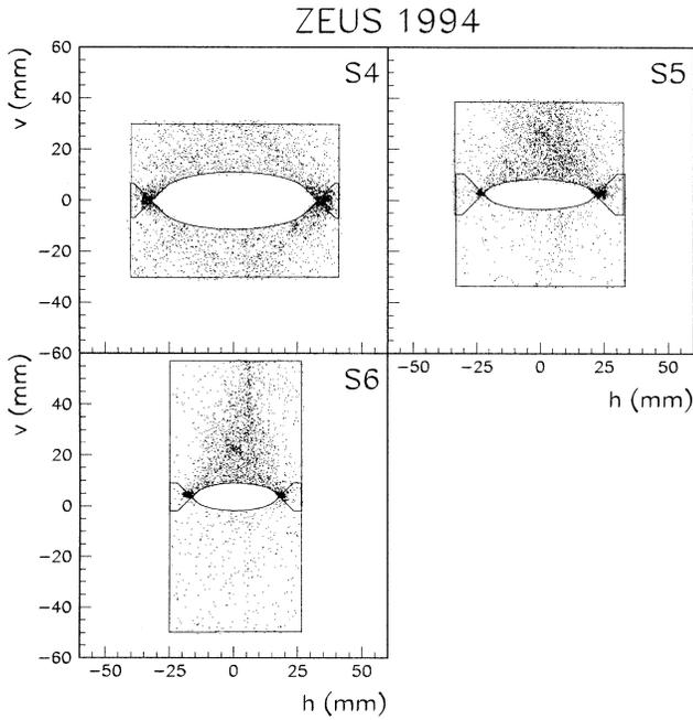
**Fig. 4.** Positions of the reconstructed track impact points in S4, S5 and S6. For each plot the origin of the reference frame coincides with the position of the nominal proton beam at the value of  $Z$  corresponding to the centre of the station. The continuous lines approximately indicate the sensitive region of the detector planes
