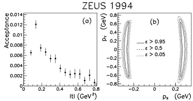
**Fig. 10.** **a** Acceptance as a function of  $t$ ; it includes the effects of the geometric acceptance of the apparatus (ZEUS and LPS), of its efficiency and resolution and of the trigger and reconstruction efficiencies. The vertical bars indicate the size of the statistical uncertainties. **b** Purely geometric acceptance  $\epsilon$  for the LPS alone for  $x_L = 1$  tracks as a function of  $p_X$  and  $p_Y$
