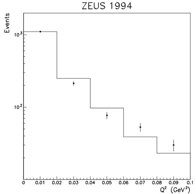
**Fig. 9.**  $Q^2$  distributions of the reconstructed data (points) and the reconstructed Monte Carlo events (histogram). The distributions are not corrected for acceptance. Only the region  $Q^2 < 0.1 \text{ GeV}^2$  is shown. The vertical bars indicate the size of the statistical uncertainties
