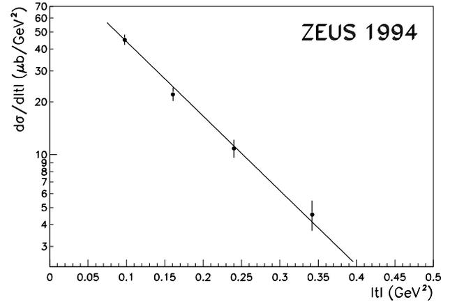
**Fig. 13.** Differential cross section  $d\sigma/d|t|$  for elastic  $\rho^0$  photoproduction,  $\gamma p \rightarrow \rho^0 p$ , at  $\langle W \rangle = 73$  GeV in the region  $0.073 < |t| < 0.40$  GeV<sup>2</sup>,  $0.55 < M_{\pi\pi} < 1.2$  GeV. The vertical bars indicate the size of the statistical uncertainties only. The line is the result of the fit described in the text
