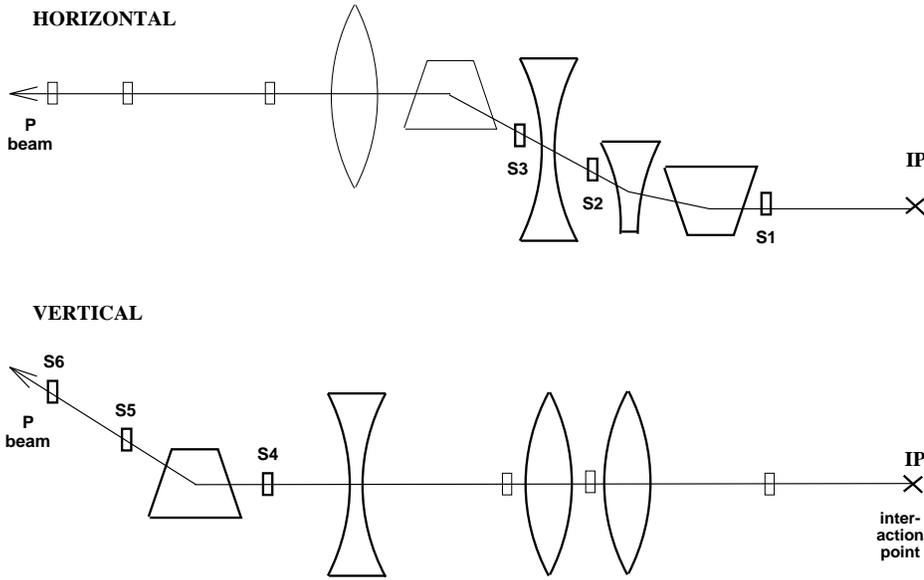
**Fig. 3.** Simplified diagram of the HERA proton beam optics relevant for the LPS. The top view (labelled “horizontal”) shows the magnetic elements relevant to the S1, S2 and S3 spectrometer as thick lines. Note the half quadrupole between S1 and S2. The side view (labelled “vertical”) shows the magnetic elements relevant to the S4, S5 and S6 spectrometer as thick lines
