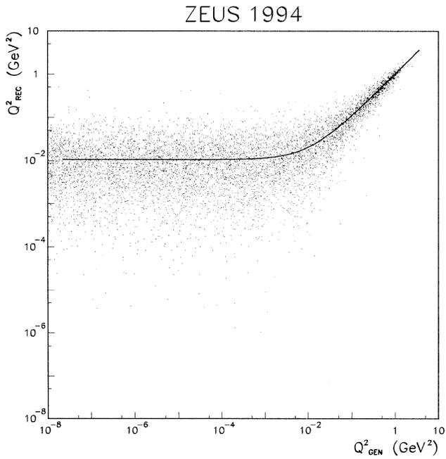
**Fig. 6.** Scatter plot of reconstructed versus generated values of  $Q^2$  for Monte Carlo events. The continuous line shows the expected average relation assuming a spread of the beam transverse momentum with standard deviations  $\sigma_{p_X} = 40$  MeV and  $\sigma_{p_Y} = 90$  MeV in the horizontal and in the vertical directions, respectively
