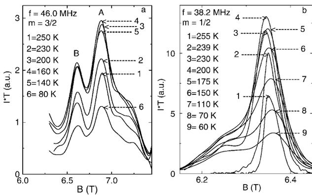
FIG. 1.  $^{139}\text{La}$  NMR field profiles for (a)  $m = 3/2$  (46.0 MHz) and (b)  $m = 1/2$  (38.2 MHz) as a function of  $T$ . Arrows point to the line maxima. For  $m = 1/2$  below 230 K a second line ( $B$ ) comes up on the low field side of line  $A$ ; for  $m = 3/2$  the two lines are visible from the start (below 250 K).
