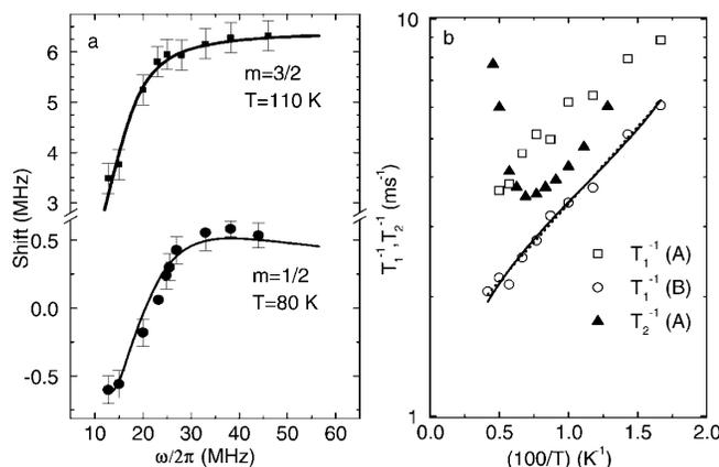
FIG. 2. (a) The position of line  $B$  as a function of resonance frequency (and hence resonance field) for  $B \parallel c$ -axis. The position of line  $A$  is field independent. The drawn line is a fit with only quadrupolar interactions. (b)  $T_1^{-1}(A)$ ,  $T_1^{-1}(B)$ , and  $T_2^{-1}(A)$  vs  $T$ . Drawn and dotted lines are, respectively, fits; see text.
