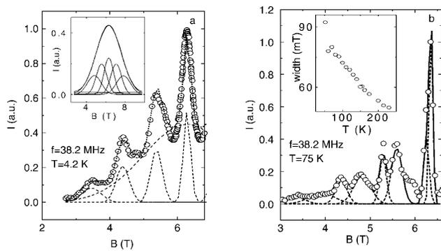
FIG. 4. Comparison of full sweeps at 4.2 K (a) and 75 K (b) shows the extra line broadening at 4.2 K. The inset in (a) shows the decomposition for the  $A$  line at 4.2 K; the inset in (b) gives the  $T$  dependence of the width of the  $A$  line for  $m = 1/2$ . Down to  $T = 60$  K the  $B$ -linewidth remains about 0.1 T (0.6 MHz).
