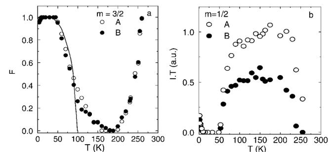
FIG. 3. (a) The  $T$  dependence of  $F$  for  $m = 3/2$ . The maximal intensities for lines  $A$  and  $B$  are both normalized to one. Drawn line is a fit to the BCS gap function. (b) Intensities ( $I$ ) times  $T$  for the decomposed  $m = 1/2$  line, divided by the maximal value of  $IT$  of line  $A$ .
