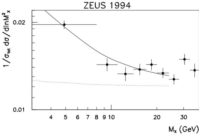
**Fig. 8.** The acceptance corrected  $M_X$  spectrum in diffractive photoproduction events fitted with the sum of a  $IPPIP$  and a  $IPPIR$  triple Regge terms (solid line). The contribution of the triple pomeron term is shown as a dotted line
