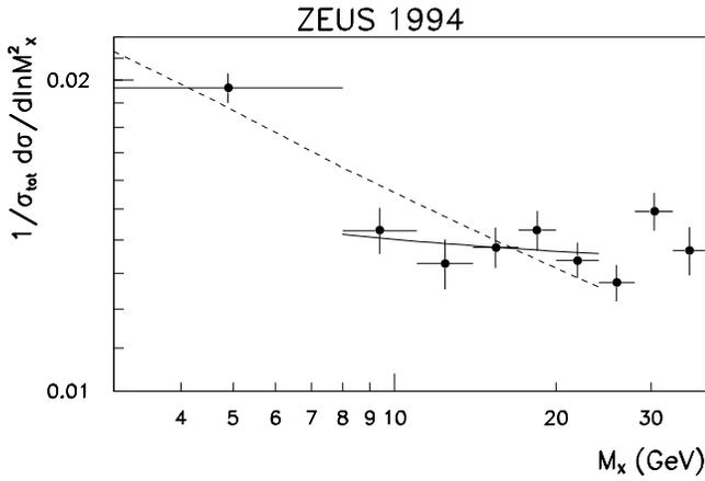
**Fig. 7.** The acceptance corrected  $M_X$  spectrum in diffractive photoproduction events. The combined statistical errors of the data and of the correction factors are shown as vertical bars. The line indicates the result of the fits of (6) to the diffractive spectrum in the intervals  $3 < M_X < 24$  GeV (dashed line) and  $8 < M_X < 24$  GeV (solid line)
