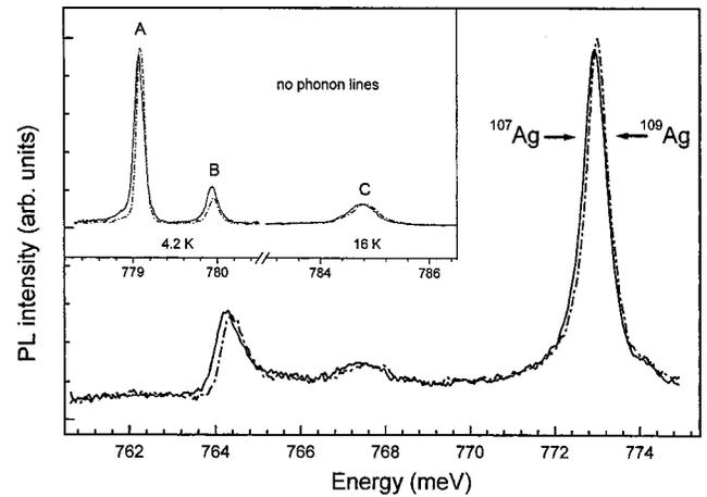
FIG. 8. Photoluminescence spectra recorded from samples doped with single isotopes of  $^{107}\text{Ag}$  or  $^{109}\text{Ag}$ . The main figure shows the effects on the one-phonon lines  $F_1$ ,  $A_1^2$ , and  $F_2$ . The inset shows the effect on the lines  $A$ ,  $B$ , and  $C$ , in agreement with Ref. 20.
