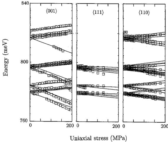
FIG. 6. The squares show the data for the splittings of the zero-phonon lines under stress along the  $\langle 001 \rangle$ ,  $\langle 111 \rangle$ , and  $\langle 110 \rangle$  crystal directions, measured in absorption at 4.2 K. The lines are the fits derived from the model described in Sec. IV.
