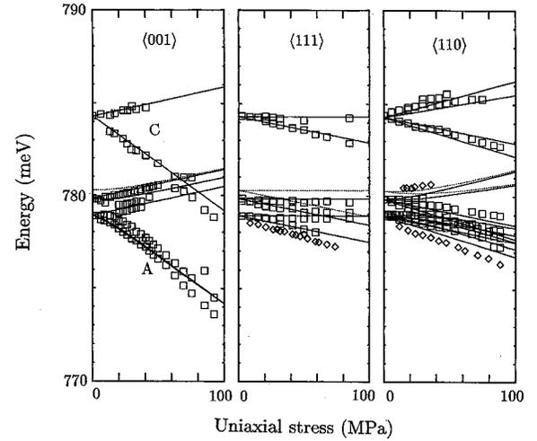
FIG. 5. The squares show the data for the splittings of the zero-phonon lines under stress along the  $\langle 001 \rangle$ ,  $\langle 111 \rangle$ , and  $\langle 110 \rangle$  crystal directions, measured in luminescence at 4.2 and 20 K. Experimental data for the transitions induced by the stresses are shown by diamonds. The lines are the fits derived from the model described in Sec. IV. Dashed lines originating near 780.2 meV show the predicted energies of the  $J=0$  state.
