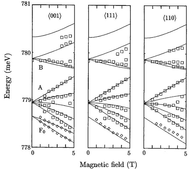
FIG. 3. The squares show the Zeeman effect measured for the zero-phonon lines A and B, and the diamonds show transitions induced from  $F_0$ . Line C, which is not shown, does not shift, as expected from the model of Sec. IV. The lines are calculated as in Sec. IV with parameters  $\lambda = -0.46$  meV,  $g_s = 1.9$ , and  $g_l = 0$ . The lines close to the data for  $F_0$  have been obtained by downshifting the fits to the lowest-energy components of line A.
