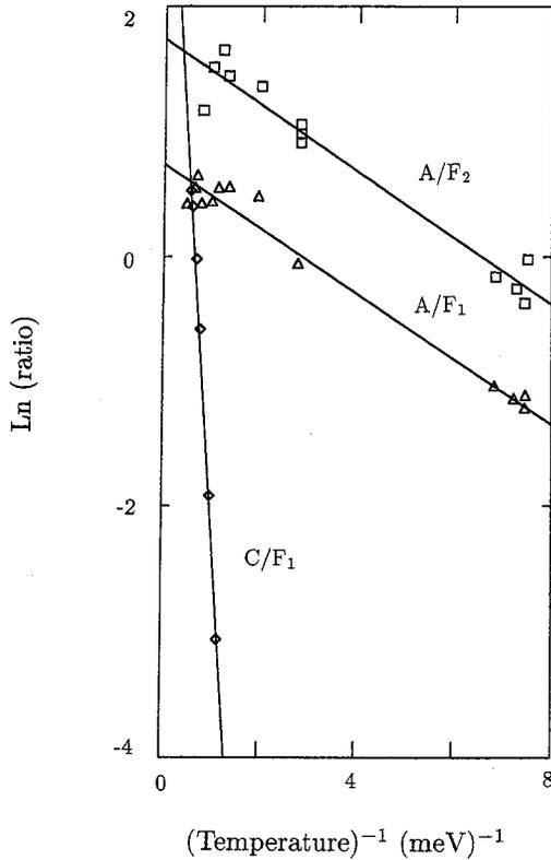
FIG. 2. Arrhenius plots of the variation with temperature of the intensities of line A relative to  $F_1$  (triangles), A relative to  $F_2$  (squares), and C relative to  $F_1$  (diamonds). Both of the activation energies for line A are  $\sim 0.26$  meV, equal to the spectroscopic separation of A from the “forbidden” line  $F_0$ , and the activation energy for line C is  $\sim 5.8$  meV, equal to the spectroscopic splitting of  $F_0$  and C.
