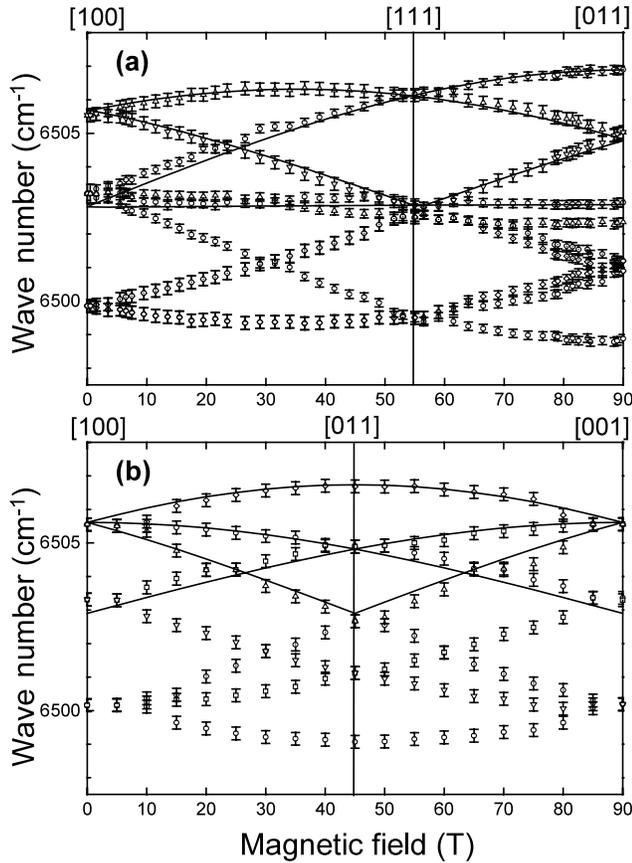
FIG. 3. Angular dependence of the Zeeman effect of the main PL line (marked with an arrow in Fig. 1) at  $B = 5.25$  T for (a) the (011) and (b) the (100) crystallographic planes. Solid lines correspond to simulations—see text for the further explanation.
