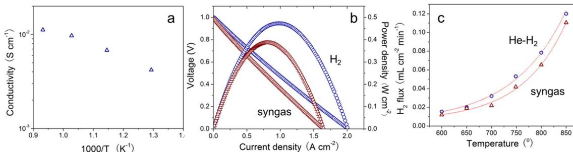
Fig. 4. (a) Arrhenius plot of the electrical conductivity of BCZYSn in humidified hydrogen; (b) polarization and power density curves of PC-SOFC in  $\text{H}_2$  and syngas at 600 °C; (c)  $\text{H}_2$  flux plots as a function of temperature using BCZYSn-GDC composite membrane, the feed gases were 50%  $\text{H}_2 + \text{He}$  and syngas, respectively.
