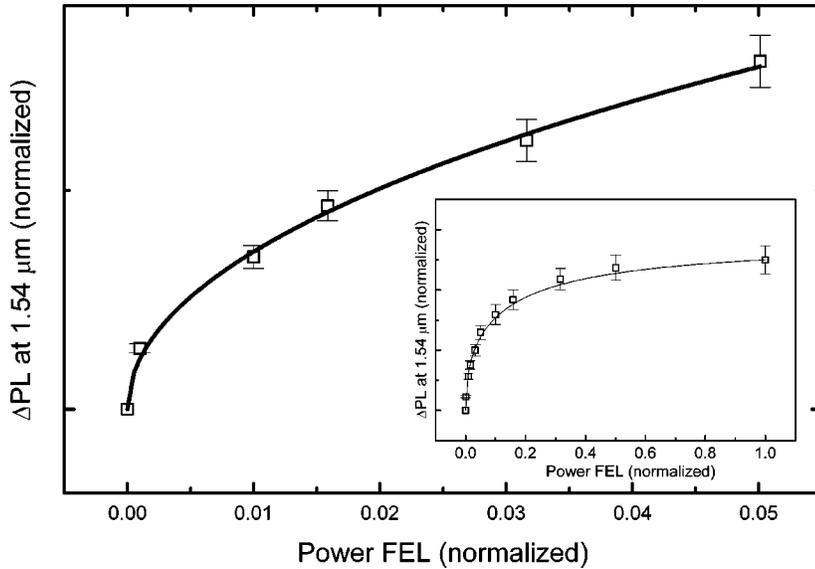
FIG. 2. Low-energy range excitation density dependence (FEL) of the MIR-induced  $\lambda \approx 1.54\text{-}\mu\text{m}$  Er emission, measured for a low-level band-to-band pumping, for  $\lambda_{\text{FEL}} \approx 10\text{ }\mu\text{m}$  and  $\Delta t = 5\text{ ms}$ . The inset shows the dependence for the full available FEL power range. The solid lines are simulations based on Eq. (27).
