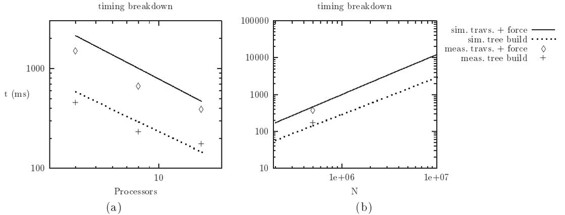
**Fig. 5.** Timings of the GDT tasks. The real system timings are also reported. The hardware architecture is a Cray T3E. (a): performance scaling with the number of processors, being  $N = 500\,000$ . (b): scaling with  $N$ , in a run with 16 processors. Note the change of scale in the two plots.
