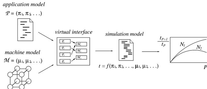
**Fig. 1.** Performance modelling process. The output of the simulation model,  $t$ , is the modelled execution time. The rightmost sketch represents a speedup graph ( $P$  is the number of processors), showing the behaviour produced by two different values assigned to a certain parameter  $N$ . The meaning of the other symbols is explained in the text.
