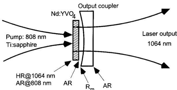
Fig. 3. Experimental setup of the microchip laser. The plano-concave configuration is longitudinally pumped by a titanium-sapphire laser at 808 nm. The crystal is  $\sim 200$   $\mu\text{m}$  thick with a refractive index of 2.2, and the air gap has a length of 0.1 mm. The radius of curvature of the output coupler is 200 mm. We can vary the reflectivity by replacing the output coupler with another one with the same radius of curvature.
