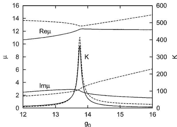
Fig. 1. Eigenvalues  $\mu$  and excess-noise factors  $K$  of the two lowest-loss transverse modes for  $\rho_g = 0.315$ . The real part of the eigenvalue corresponds to the phase shift per Rayleigh range; the imaginary part, to the modal gain. For fixed gain width  $\rho_g$  and gain strength  $g_0 \rightarrow 0$ , the modes are adiabatically connected to mode  $u_2$  (solid curves) and  $u_3$  (dashed curves) of the parabolic index guide; see also Fig. 2.
