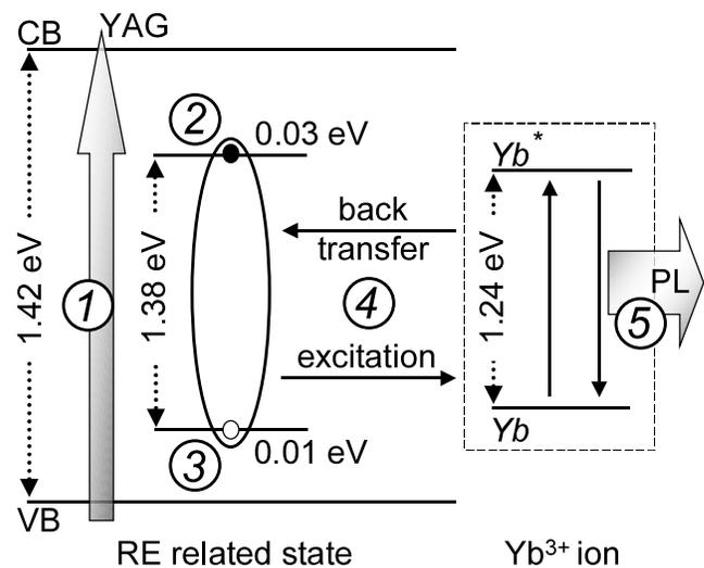
FIG. 1. Model of excitation of  $\text{Yb}^{3+}$  in InP. After band-to-band excitation (1) the generated free electrons can be captured at the Yb related trap (2). Binding of a hole (3) forms an electron-hole pair on the trap. Nonradiative recombination of the pair leads to excitation of the  $\text{Yb}^{3+}$  ion (4), producing the observed PL (5).
