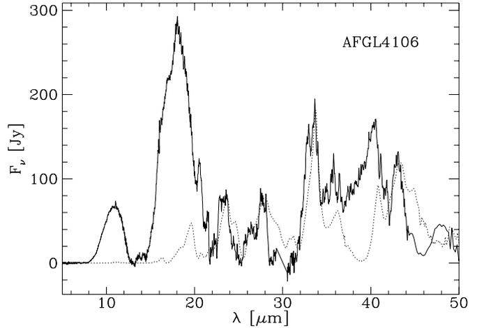
**Fig. 16.** A fit (dotted line) to the continuum subtracted spectrum (solid line) of AFGL 4106.  $T_f = 100$  K and  $T_e = 80$  K. Note, that we made no attempt to fit the amorphous silicate bands in the continuum subtracted spectrum.
