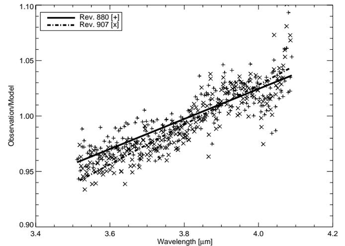
**Fig. 6.** Division of the observed spectrum of  $\gamma$  Draconis by a synthetic spectrum in the beginning and the end of the post-helium phase. The Relative Spectral Response of the SWS tilts more as the temperature increases.
