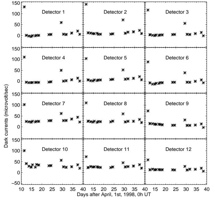
**Fig. 5.** The variation of the mean detector dark signals during the post-helium phase.
