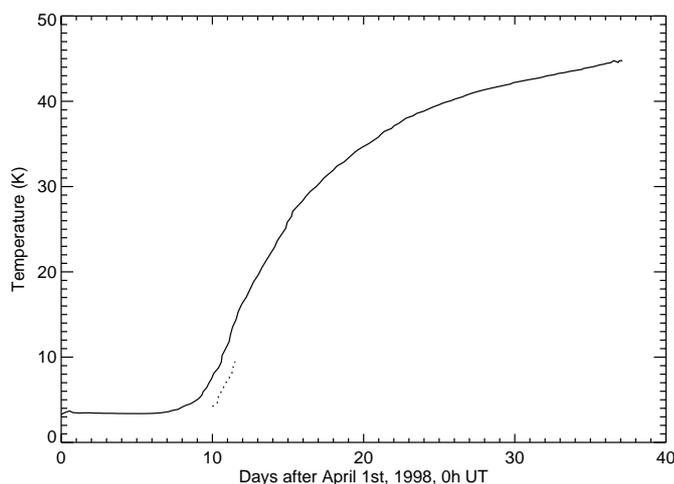
**Fig. 2.** The temperatures of the optical support structure (lower short curve, dashes) and of the upper baffle of the ISO telescope (upper curve, solid line) increased smoothly during the post-He phase.
