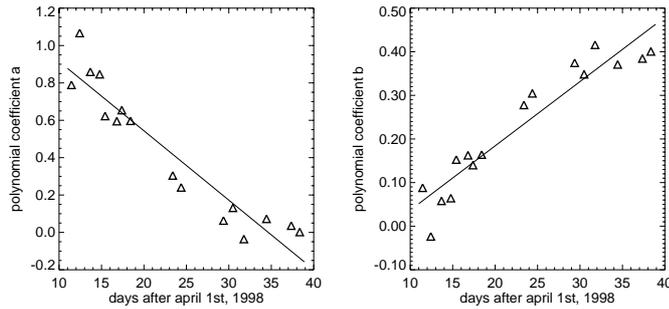
**Fig. 7.** Characterisation of the changing slope of the RSRF for detector 7 in AOT-band 1A. The triangles are the polynomial coefficients of the fits to the slope difference between calibration observations and model spectra. The solid line is a linear fit to the coefficients against time.
