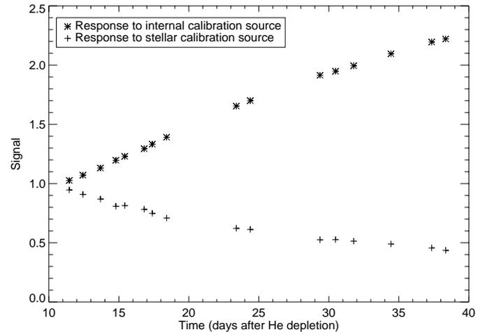
**Fig. 8.** Change of the SWS detector 7 response to the signal of the internal calibration source and to the signal of an external calibration star.
