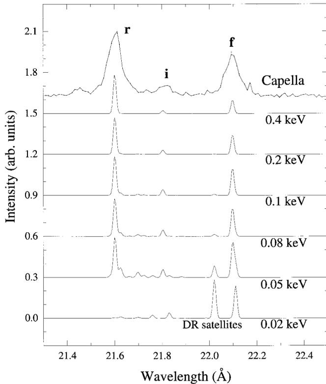
**Fig. 3.** Observed O VII triplet with calculated spectra of the O VII and O VI DR satellite lines for six different electron temperatures. The plots are normalized to the strongest line in each spectrum. Note the steep temperature sensitivity of the DR satellites (see text)
