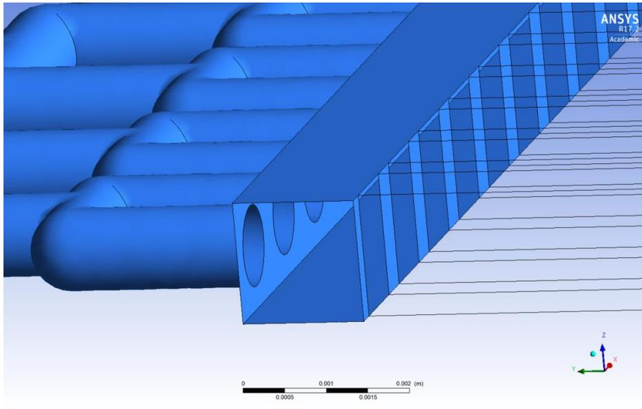
Figure 1S. A zoom-in of the design used for the simulation. The walls of the distributor and the  $1^{\text{D}}$  channel are with blue, while the walls of the  $2^{\text{D}}$  channels are shown as a wireframe.
