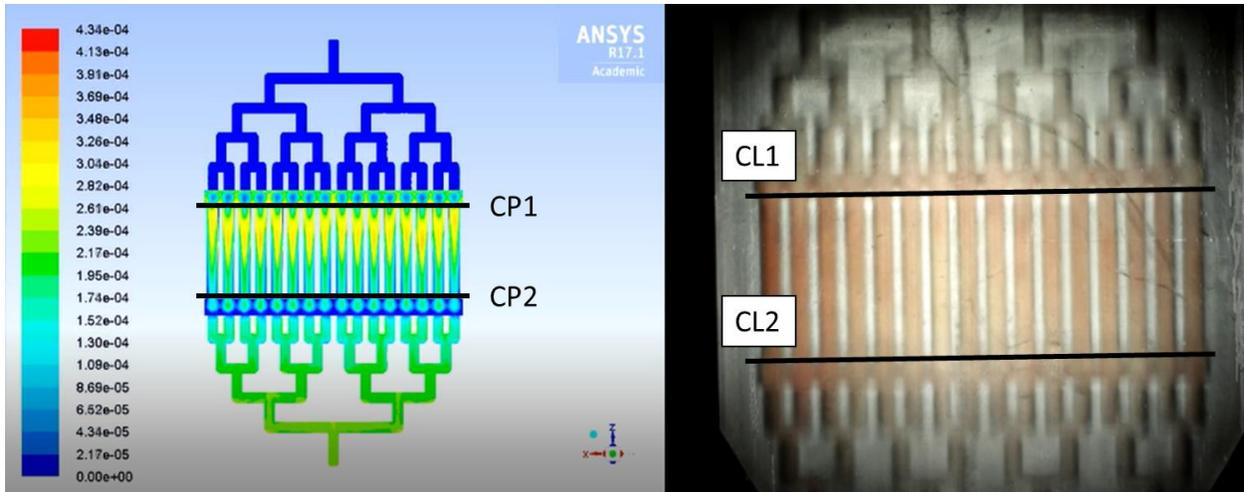
Figure 2S. Left: the profile of the mass fraction of dye calculated via computational fluid dynamics (CFD), right: the red dye migrating in the device.
