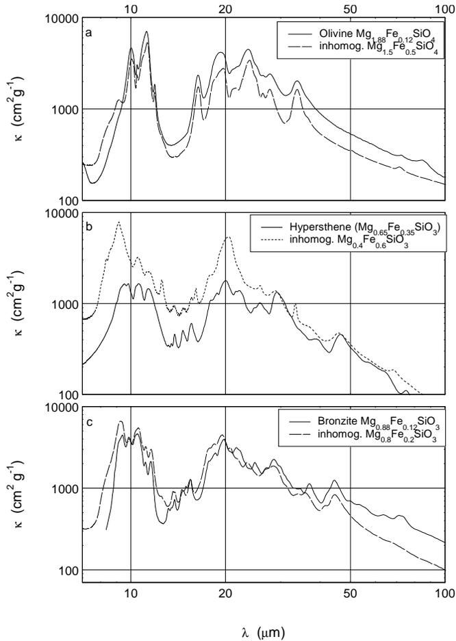
**Fig. 6.** **a** and **b** show a comparison of the mass absorption coefficients for two inhomogeneous synthetic samples (see Fig. 1 and Table 2) of olivine and pyroxene composition, respectively, with the corresponding homogeneous materials. **c** presents another inhomogeneous pyroxene sample with a composition more similar to the homogeneous bronzite material, which shows a good agreement between the two spectra.
