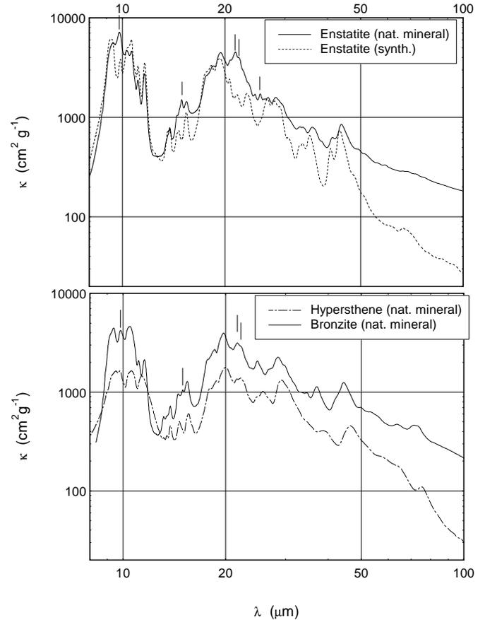
**Fig. 3.** Mass absorption coefficients calculated from transmission spectra for different pyroxene minerals. The vertical strokes mark the peaks which are superimposed by the  $\text{Mg}_3[(\text{OH})_2/\text{Si}_4\text{O}_{10}]$  (talc) phase.
