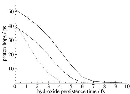
**Figure 6.17:** Number of observed proton hops per ps per proton hole as function of the persistent lifetime of the resulting hydroxide ion for the concentrated (solid line) and dilute (dashed line) LiOH solution. For comparison we also plotted the same quantity for the reference solution of one OH<sup>-</sup> ion in water (dotted line).
