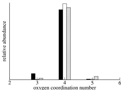
**Figure 6.4:** Histograms of the coordination number based on the Li-O distance for the concentrated (filled bars), dilute (open bars) and reference solution (dot-filled bars).
