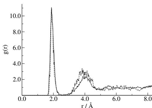
**Figure 6.5:**  $\text{Li-OH}^-$  radial distribution functions for the dilute (dashed line) and concentrated (solid line) solution.
