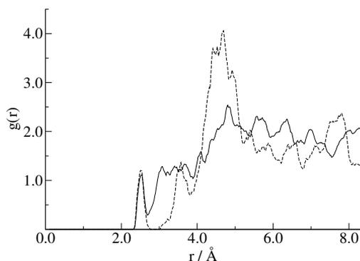
**Figure 6.13:**  $\text{OH}^-$ – $\text{OH}^-$  radial distribution functions for the dilute (dashed line) and concentrated (solid line) solution.
