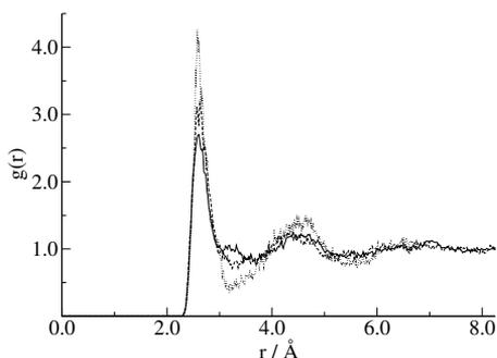
**Figure 6.11:** O-OH<sup>-</sup> radial distribution functions for the dilute (dashed line) and concentrated (solid line) solution. The dotted line represents the O-OH<sup>-</sup> RDF for the reference system of a single hydroxide ion in water.
