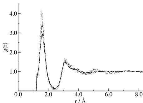
**Figure 6.12:** H-OH<sup>-</sup> radial distribution functions for the dilute (dashed line) and concentrated (solid line) solution. The dotted line represents the H-OH<sup>-</sup> RDF for the reference system of a single hydroxide ion in water.
