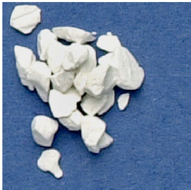
Figure 2 Samples of the granule types illustrate the differences in shape and macro-porosity: Allogran
