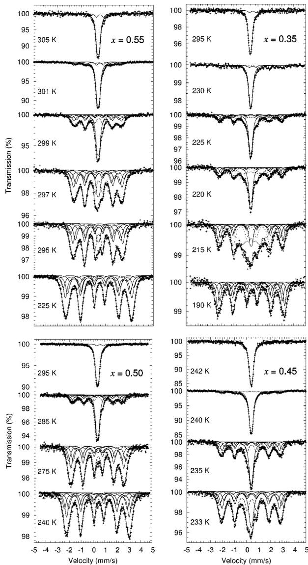
FIG. 2. The Mössbauer spectra of  $\text{FeMnP}_{1-x}\text{As}_x$ , where  $x = 0.35, 0.45, 0.50,$  and  $0.55$ , going clockwise from  $x = 0.35$  in the upper right-hand side panel. The dashed line is the sum of the ferromagnetic components. For  $x = 0.35$ , the dotted line is the sum of the antiferromagnetic components. The small doublet in the paramagnetic spectra, for  $x = 0.35, 0.50,$  and  $0.55$ , corresponds to iron on the pyramidal manganese site.
