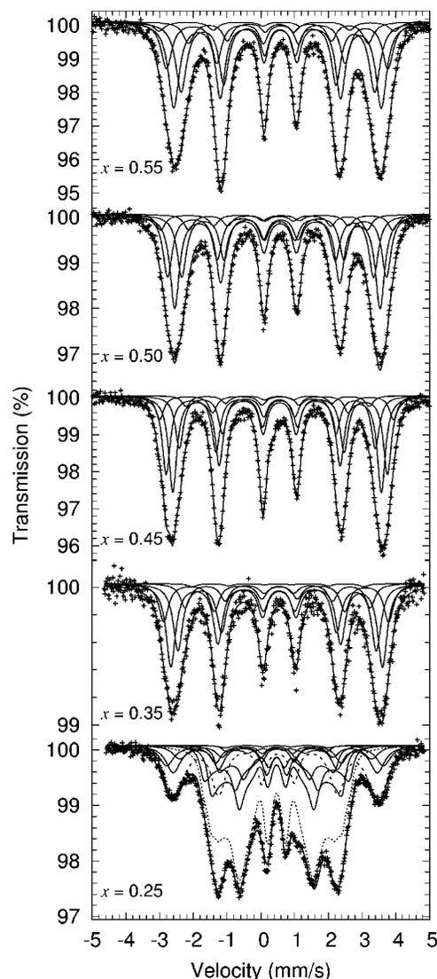
FIG. 1. The Mössbauer spectra of  $\text{FeMnP}_{1-x}\text{As}_x$  obtained at 4.2 K. For  $x=0.25$  the dashed and the dotted lines are the sum of the binomial ferromagnetic and antiferromagnetic components, respectively.
