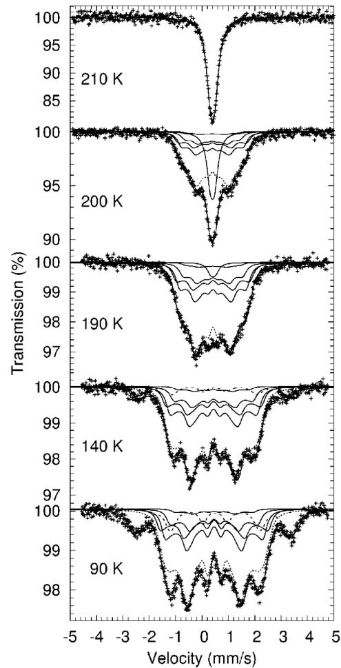
FIG. 3. The Mössbauer spectra of  $\text{FeMnP}_{0.75}\text{As}_{0.25}$  obtained at the indicated temperatures. The dashed and dotted lines are the sum of the ferromagnetic and antiferromagnetic components, respectively. The weakest antiferromagnetic component assigned to the iron with four arsenic near neighbors is not shown.
