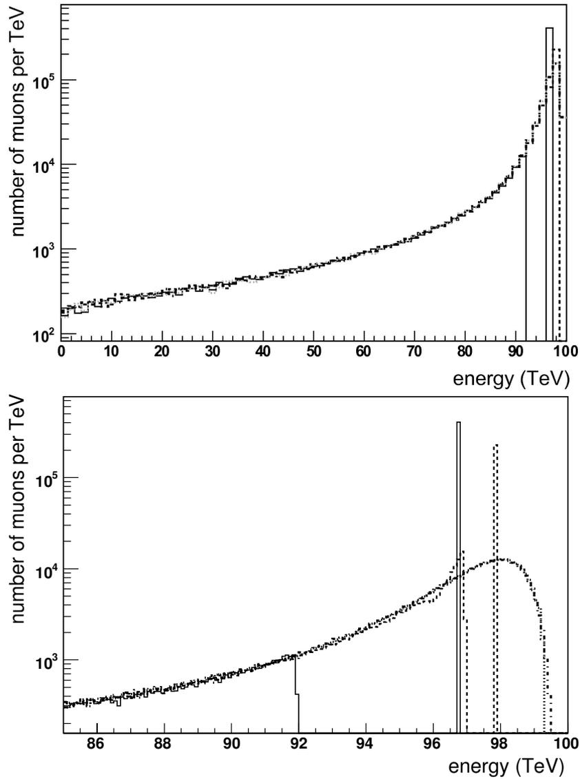
Figure B.1: Comparison of the final energy distributions of  $10^7$  muons with initial energy 100 TeV which were propagated through 300 meters of ANTARES Water, calculated by MMC with an energy cutoff  $v_{cut} = 0.05$  (solid line),  $v_{cut} = 0.01$  (dashed),  $v_{cut} = 10^{-3}$  (dotted) and  $v_{cut} = 10^{-4}$  (dashed-dotted). On the right is a close-up on the left figure.
