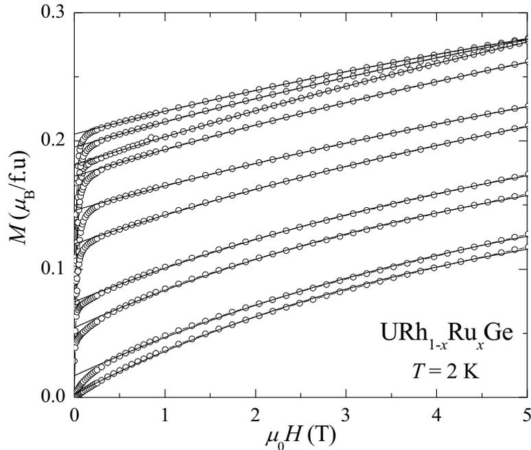
Figure 4.8 Field dependence of the magnetization of  $\text{URh}_{1-x}\text{Ru}_x\text{Ge}$  alloys measured in a field up to 5 T at 2 K. The solid lines represent fits to Eq. 4.3. Ru concentrations are (from top to bottom)  $x = 0.05, 0.1, 0, 0.15, 0.2, 0.25, 0.3, 0.325, 0.35$  and  $0.4$ .
