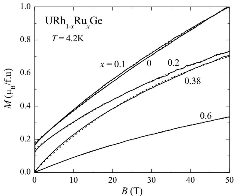
Figure 4.9 High-field magnetization of  $\text{URh}_{1-x}\text{Ru}_x\text{Ge}$  alloys measured in a field up to 50 T at 4.2 K. The dotted lines indicate fits to Eq. 4.3. Ru concentrations are (from top to bottom)  $x = 0.1, 0, 0.2, 0.25, 0.38$  and  $0.6$ .
