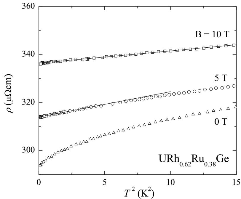
Figure 4.13 The resistivity of URh<sub>0.62</sub>Ru<sub>0.38</sub>Ge at different magnetic fields plotted versus  $T^2$ . The fields (oriented perpendicular to the current) are (from bottom to top)  $B = 0, 5$  and 10 T. The lines represent fits of the data to  $\rho \sim T^2$ .
