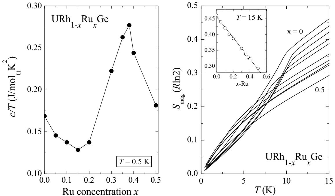
Figure 4.16 *Left panel*: The  $\gamma$  value at  $0.5$  K as a function of Ru concentration. *Right panel*: The magnetic entropy  $S_{\text{mag}}$  (in units of  $R \ln 2$ ) for  $\text{URh}_{1-x}\text{Ru}_x\text{Ge}$  alloys with  $0 \leq x \leq 0.5$ . *Inset*: Concentration dependence of  $S_{\text{mag}}$  at a fixed temperature of  $15$  K.
