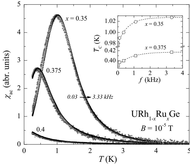
Figure 4.17 Temperature dependence of the ac-susceptibility in  $URh_{1-x}Ru_xGe$  for  $x = 0.35$ , 0.375 and 0.4 at frequencies  $f = 0.03, 0.11, 0.35, 1.11$  and 3.33 kHz. The data are scaled to the maximum amplitude of  $\chi_{ac}$  at 3.33 kHz using multiplication factors of  $1 \pm 0.03$  for  $f = 0.11, 0.35$  and 1.11 kHz and  $\sim 1.2$  for  $f = 0.03$  kHz. The inset shows  $T_C(f)$ .
