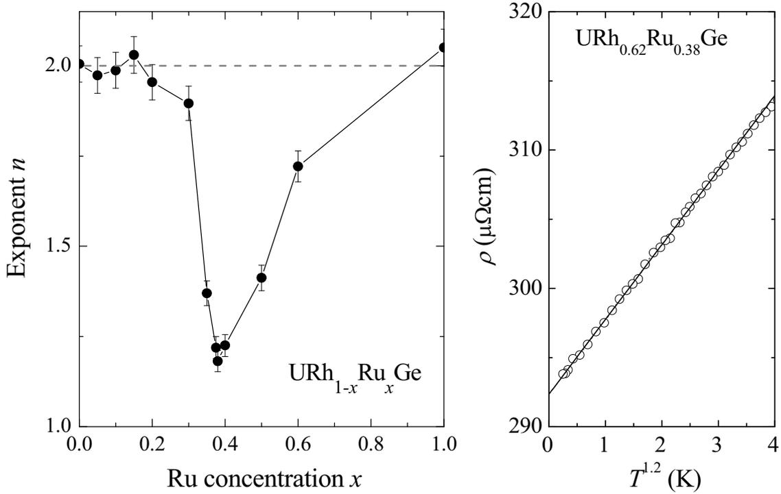
Figure 4.12 Left panel: The exponent  $n$  of the  $\rho \sim T^n$  term in the electrical resistivity of  $\text{URh}_{1-x}\text{Ru}_x\text{Ge}$  alloys versus Ru concentration. The horizontal dashed line indicates  $n = 2$ . Right panel: The resistivity of  $\text{URh}_{0.62}\text{Ru}_{0.38}\text{Ge}$  versus  $T^{1.2}$ . The solid line represents a fit of the data to  $\rho \sim T^{1.2}$ .
