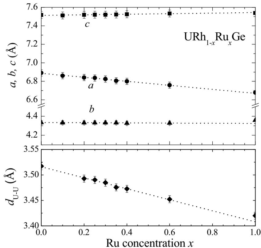
Figure 4.3 Upper frame: Lattice parameters of  $\text{URh}_{1-x}\text{Ru}_x\text{Ge}$  as a function of the Ru concentration  $x$  measured at room temperature. Lower frame: The shortest Uranium-Uranium distance of  $\text{URh}_{1-x}\text{Ru}_x\text{Ge}$  as a function of the Ru concentration  $x$ . Data for  $\text{URuGe}$  are taken from Ref.[39].
