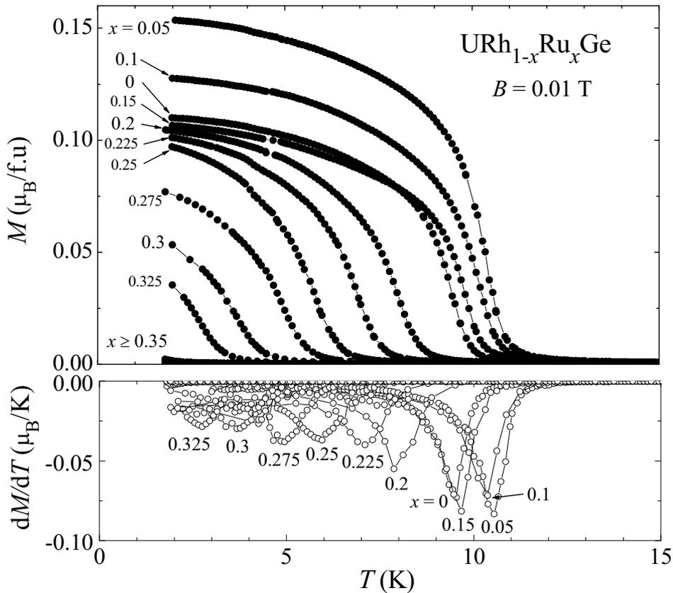
Figure 4.4 Upper frame: Temperature variation of the dc magnetization measured in a field  $B = 0.01$  T of URh<sub>1-x</sub>Ru<sub>x</sub>Ge alloys. Notice  $T_C$  first increases and has a maximum value for  $x = 0.05$ . For  $0.35 \leq x \leq 1$  magnetic order is not observed above  $T = 1.8$  K. The solid lines connect the data points. Lower frame: Temperature derivative of the magnetization.
