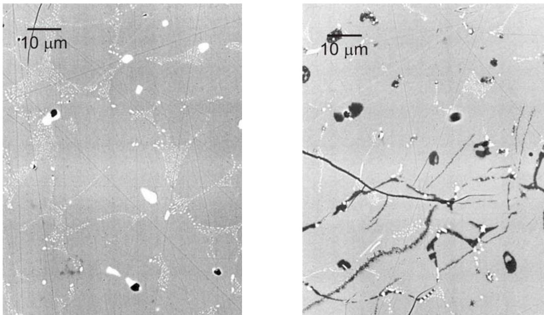
Figure 4.2 EPMA micrographs of  $URhGe$  (left panel) and  $URh_{0.8}Ru_{0.2}Ge$  (right panel). The grey areas represent the main matrix. The (big and small) light spots are the Uranium rich phases. The black spots and black lines are holes and cracks on the surface, respectively.
