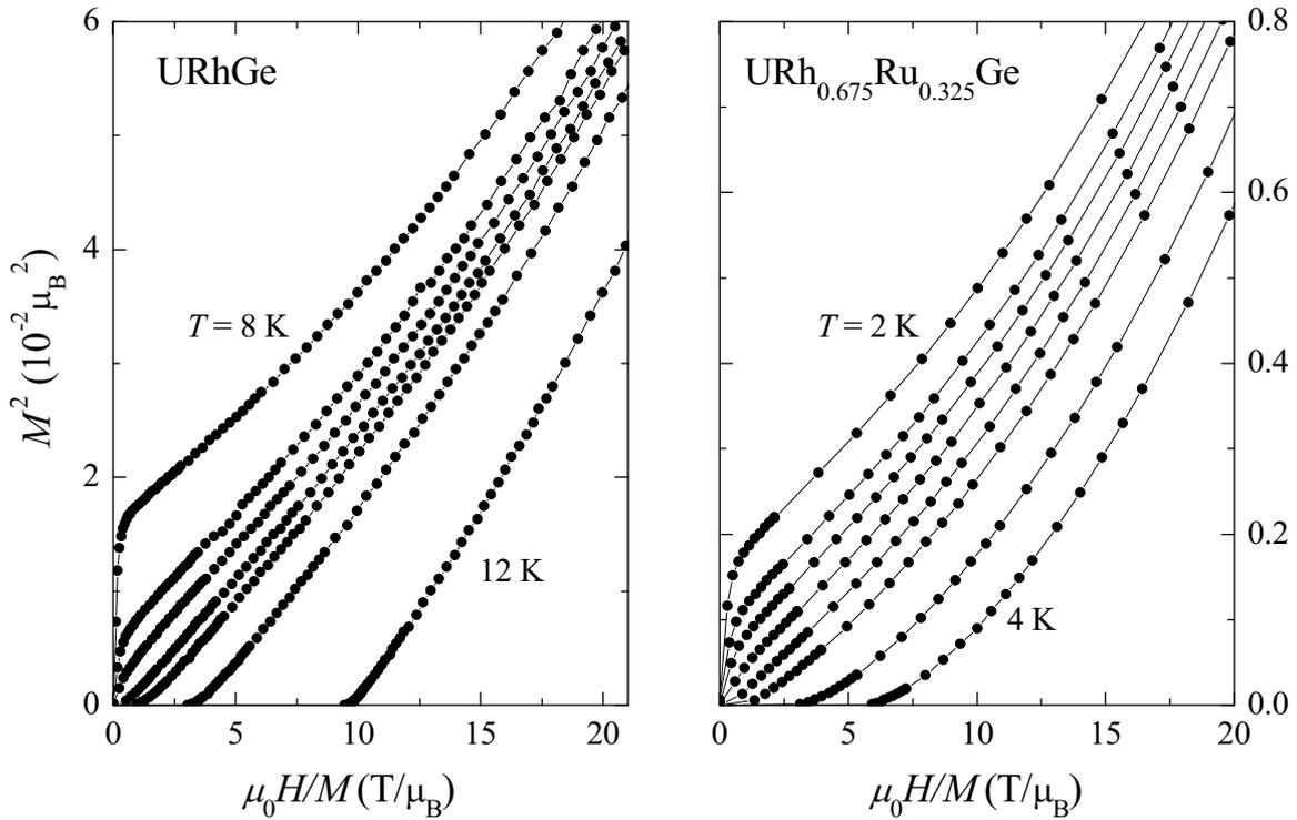
Figure 4.5 Arrott plots of the magnetization of (*left panel*) URhGe with the isotherms measured (from top to down) at  $T = 8.0, 9.2, 9.5, 9.8, 10.0, 10.5$  and  $12.0$  K and (*right panel*) URh<sub>0.675</sub>Ru<sub>0.325</sub>Ge with the isotherms measured (from top to down) at  $T = 2.0, 2.4, 2.6, 2.8, 3.0, 3.2, 3.6$  and  $4.0$  K. The isotherm through the origin determines  $T_C = 9.6$  and  $2.8$  K for URhGe and URh<sub>0.675</sub>Ru<sub>0.325</sub>Ge, respectively.
