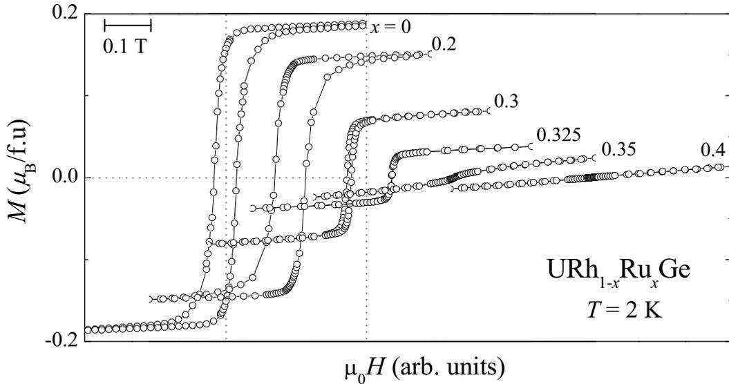
Figure 4.6 Hysteresis loops of  $\text{URh}_{1-x}\text{Ru}_x\text{Ge}$  alloys measured at the temperature of 2 K. The bar gives an absolute field scale. Ru concentrations are (from left to right)  $x = 0, 0.2, 0.3, 0.325, 0.35$  and  $0.4$ .
