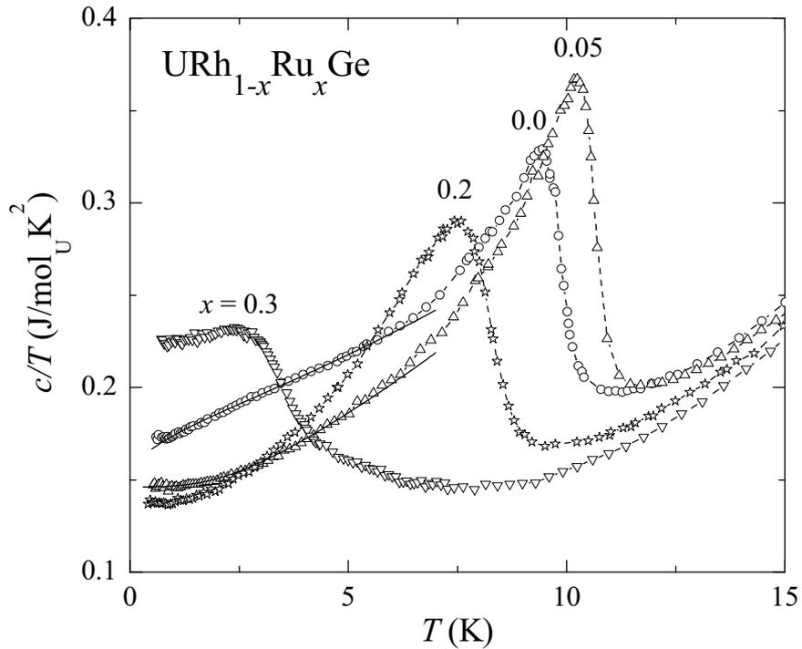
Figure 4.14 Low-temperature specific heat in a plot of  $c/T$  versus  $T$  of selected  $\text{URh}_{1-x}\text{Ru}_x\text{Ge}$  alloys with  $x \leq 0.3$ . The solid lines represent fits to Eq. 4.7 and Eq. 4.8 (with addition of the lattice contribution) for  $x = 0$  and  $x = 0.05$ , respectively.
