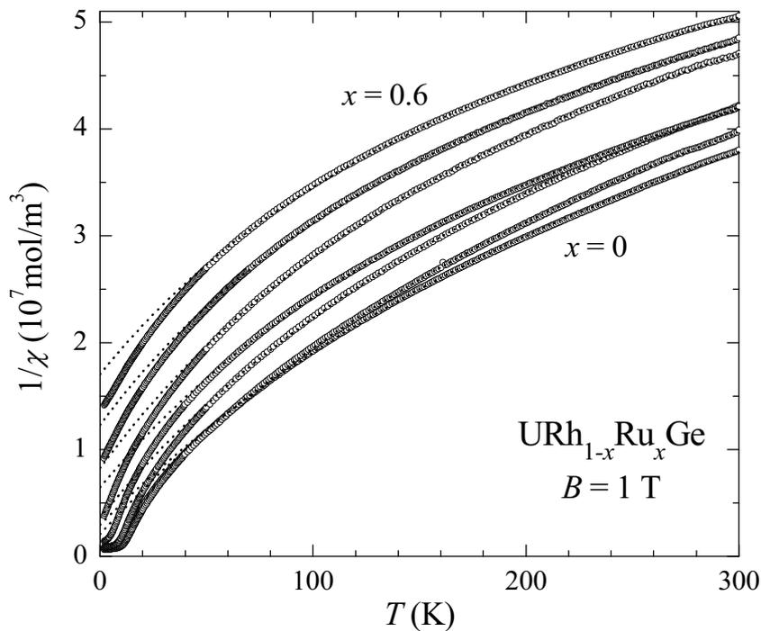
Figure 4.7 Temperature variation of the inverse susceptibility  $1/\chi$  of selected  $\text{URh}_{1-x}\text{Ru}_x\text{Ge}$  alloys measured in a field of 1 T. The dotted lines are the best fits to the MCW law in the temperature range  $T = 50 - 300$  K. Ru concentrations are (from bottom to top)  $x = 0, 0.1, 0.2, 0.3, 0.4, 0.5$  and  $0.6$ .
