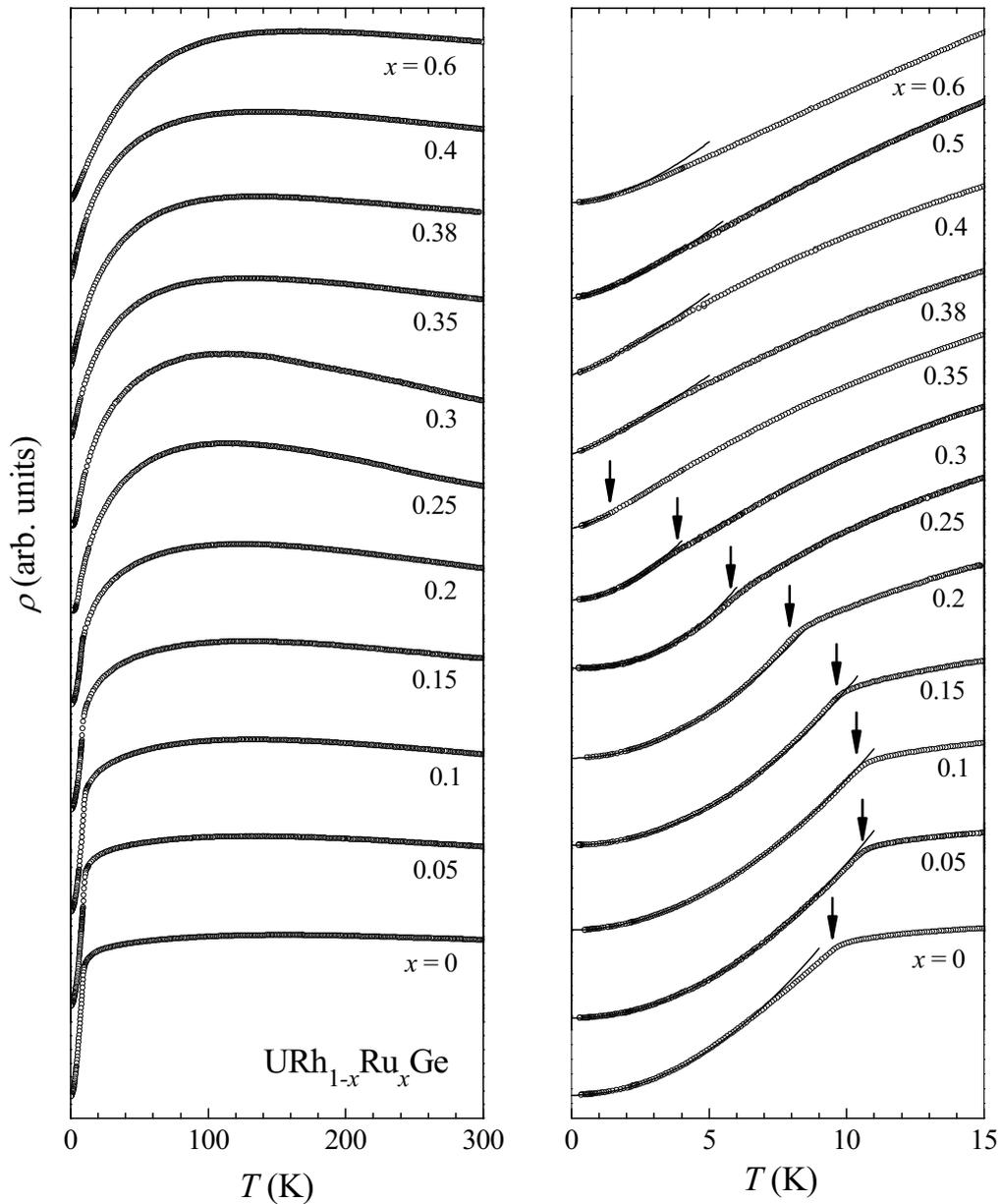
Figure 4.11 Temperature dependence of the electrical resistivity  $\rho$  in arbitrary units of  $URh_{1-x}Ru_xGe$  alloys for  $0 \leq x \leq 0.6$  as indicated. *Left panel:*  $2 \text{ K} \leq T \leq 300 \text{ K}$ . *Right panel:*  $0.25 \text{ K} \leq T \leq 15 \text{ K}$ . The Curie temperatures are indicated by arrows. The solid lines are fits to Eq. 4.5.
