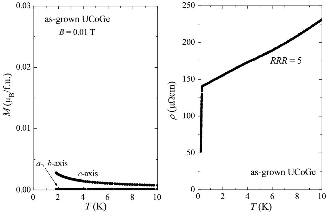
Figure 7.15 Left panel: Magnetization as a function of temperature in a field  $B$  of 0.01 T applied along the principal axes of as-grown single-crystalline UCoGe as indicated. Right panel: Temperature dependence of the electrical resistivity measured on as-grown single-crystalline UCoGe with  $RRR \approx 5$ . (As the crystal was not oriented the direction of the current is not specified).
