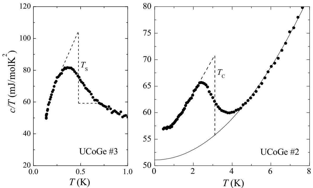
Figure 7.6 Temperature dependence of the specific heat of UCoGe divided by temperature  $c/T$  in zero field. The solid line represents an estimate of the lattice contribution together with an electronic term of  $50.4 \text{ mJ/molK}^2$ . *Left panel:*  $c/T$  in the temperature range 0.1 - 1 K measured on sample #3. *Right panel:*  $c/T$  in  $T > 0.5 \text{ K}$  measured on sample #2.
