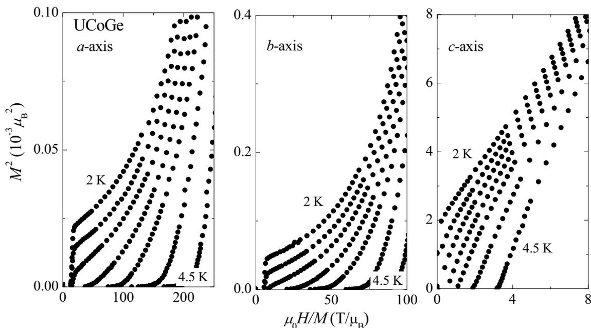
Figure 7.18 Arrott plots of the magnetization of single-crystalline UCoGe with the isotherms measured (from top to down) at  $T = 2, 2.4, 2.7, 3.0, 3.3, 3.8$  and 4.5 K. The isotherm through the origin determines  $T_C = 2.8$  K. Notice the different horizontal and vertical scales.
