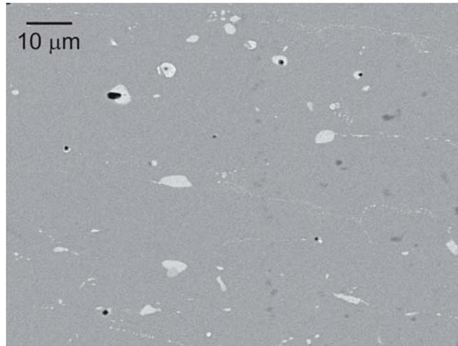
*Figure 7.1* EPMA micrograph of UCoGe (sample #3). The grey area represents the main matrix UCoGe. The (big and small) light spots are Uranium rich phases, while the dark grey spots are Uranium poor phases. The black spots are holes on the surface.
