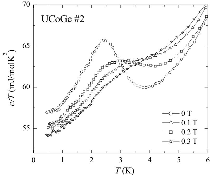
Figure 7.7 The temperature dependence of the specific heat of UCoGe (sample #2) plotted as  $c/T$  versus  $T$  in fields of 0, 0.1, 0.2 and 0.3 T.
