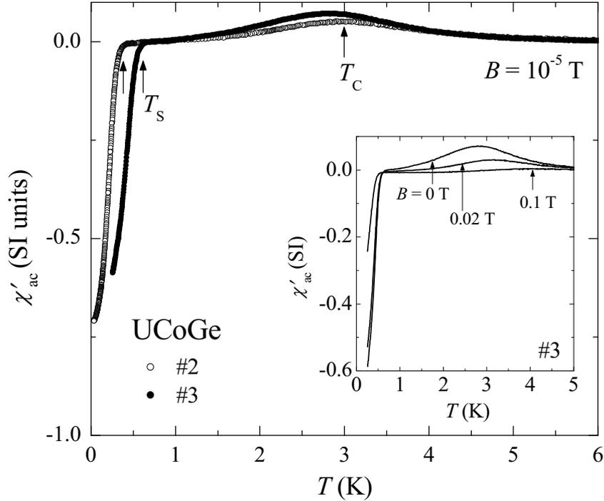
Figure 7.5 Temperature dependence of the real part of the ac-susceptibility  $\chi'_{ac}$  in polycrystalline UCoGe (samples #2 and #3). Arrows indicate  $T_C$  and  $T_S$ . *Inset*: The ac-susceptibility of sample #3 measured in fields of 0, 0.02 and 0.1 T.
