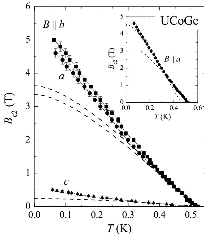
Figure 7.21 Temperature dependence of the upper critical field of UCoGe for  $B$  along the principal axes. The dashed lines show the calculated dependence for a superconducting gap function with axial (along  $c$  axis) and polar symmetries (along  $a$  and  $b$  axis) (see text). Inset:  $B_{c2}(T)$  for  $B \parallel a$ , plotted together with the polar state functions for two superconducting phases with zero-field transitions at 0.46 and 0.52 K.
