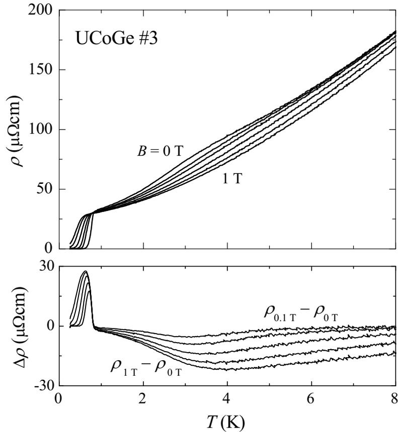
Figure 7.4 The temperature dependence of the resistivity of polycrystalline UCoGe (sample #3) in applied fields of 0, 0.1, 0.2, 0.4, 0.7 and 1 T (upper frame) and  $\Delta\rho$  obtained by subtracting of the zero-field resistivity from the resistivity measured in applied field (lower frame).
