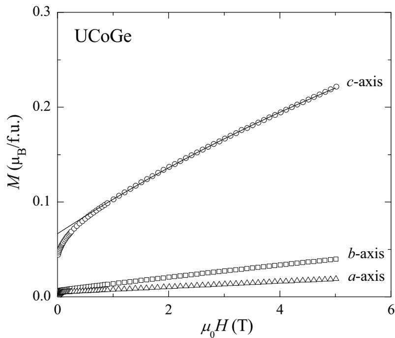
Figure 7.19 Field dependence of the magnetization of single crystalline UCoGe measured in a field up to 5 T along the  $a$ ,  $b$  and  $c$  axis at 2 K. The solid line for  $B \parallel c$  represents a fit to Eq. 4.3.
