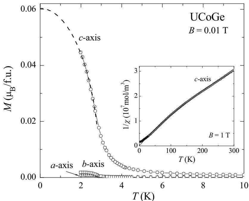
Figure 7.17 Magnetization as a function of temperature in a field  $B$  of 0.01 T applied along the principal axes of annealed UCoGe as indicated. The dashed line presents the fit to the relation  $M(T)^2 = M_0^2(1 - (T/T^*)^2)$  (see text). *Inset:* Temperature variation of the reciprocal susceptibility of UCoGe single-crystal measured in a field of 1 T. The solid line is the best fit to a MCW law in the temperature range 50 - 300 K.
