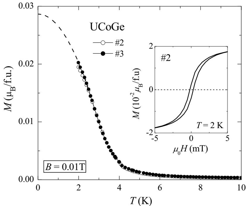
Figure 7.2 Magnetization of UCoGe (samples #2 and #3) as a function of temperature in a field  $B$  of 0.01 T as indicated. The dashed line is a smooth extrapolation of the data for sample #3 to 0 K. *Inset*: Hysteresis loop measured for sample #2 at 2 K in the FM state.
