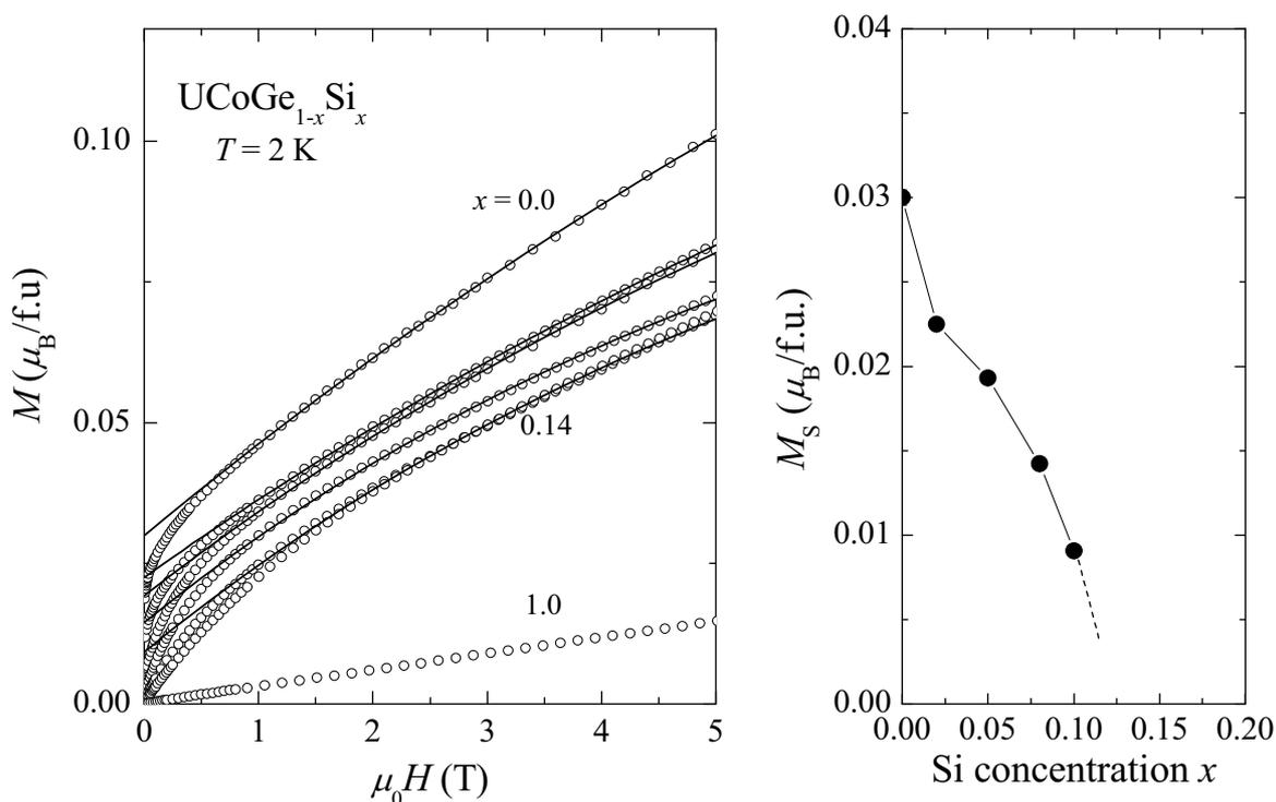
Figure 8.4 Left panel: Field dependence of the magnetization of  $\text{UCoGe}_{1-x}\text{Si}_x$  alloys measured in a field up to 5 T at 2 K. The solid lines represent fits to Eq. 4.3 for the ordered compounds. Si concentrations are (from top to bottom)  $x = 0, 0.02, 0.05, 0.08, 0.1, 0.14$  and 1. Right panel: The spontaneous moment  $M_S$  of  $\text{UCoGe}_{1-x}\text{Si}_x$  as a function of Si concentration.
