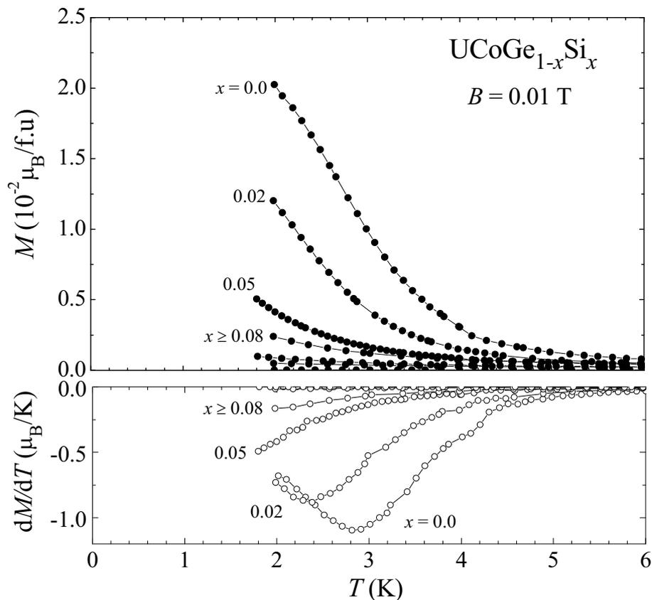
Figure 8.2 Upper frame: Temperature variation of the dc-magnetization measured in a field  $B = 0.01 \text{ T}$  of  $\text{UCoGe}_{1-x}\text{Si}_x$ . For  $x \geq 0.05$  the Curie temperature could not be determined from the data. Lower frame: Temperature derivative of the magnetization.
