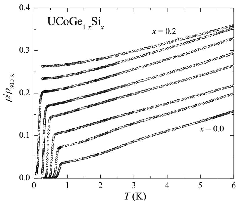
Figure 8.6 Temperature dependence of the electrical resistivity divided by the resistivity at room temperature  $\rho/\rho_{\text{RT}}$  of  $\text{UCoGe}_{1-x}\text{Si}_x$  for  $0 \leq x \leq 0.2$ . Si concentrations are (from bottom to top)  $x = 0, 0.02, 0.04, 0.06, 0.08, 0.1, 0.14$  and  $0.2$ .
