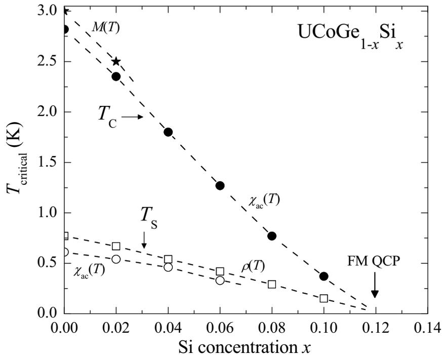
Figure 8.9 Temperature-composition phase diagram  $T(x)$  of  $\text{UCoGe}_{1-x}\text{Si}_x$ . The Curie temperature  $T_C$  and the superconducting transition temperature  $T_S$  are determined from  $M(T)$ ,  $\rho(T)$  and  $\chi_{ac}(T)$ . The dashed lines serve to guide the eye.
