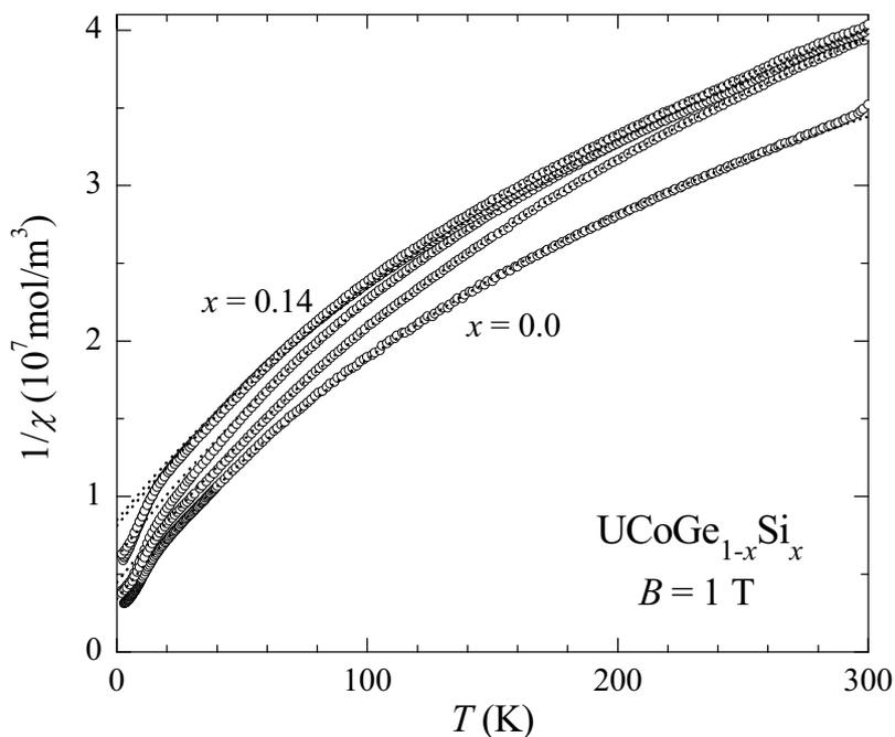
Figure 8.5 Temperature variation of the reciprocal susceptibility of  $\text{UCoGe}_{1-x}\text{Si}_x$  alloys measured in a field of 1 T. The dotted lines are the best fits to the MCW law in the temperature range  $T = 50 - 300\text{ K}$ . Notice for  $x = 0.1$  the data is plotted down to 50 mK.
