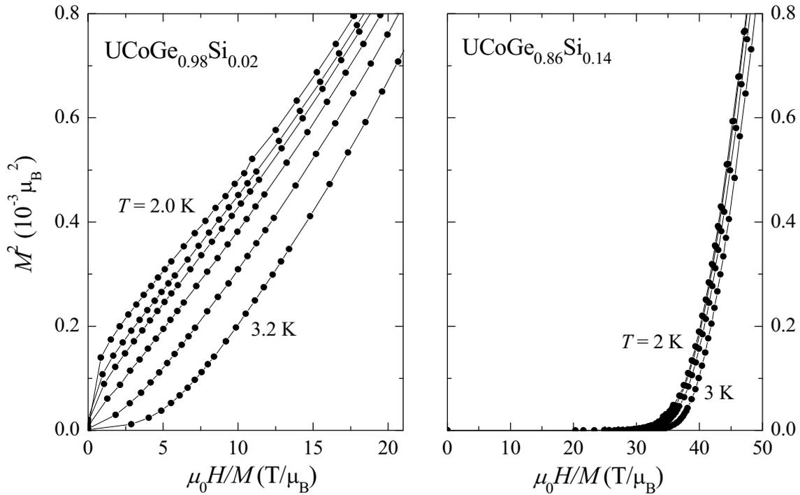
Figure 8.3 Arrott plots of the magnetization of  $UCoGe_{1-x}Si_x$  alloys. *Left panel:*  $x = 0.02$  with isotherms measured (from top to bottom) at  $T = 2.0, 2.2, 2.3, 2.5, 2.7$  and  $3.2 \text{ K}$ . *Right panel:*  $x = 0.14$  with isotherms measured (from top to bottom) at  $T = 2.0, 2.2, 2.5$  and  $3.0 \text{ K}$ . The isotherm through the origin determines  $T_C = 2.5 \text{ K}$  for  $x = 0.02$ . The ground state for  $x = 0.14$  is paramagnetic.
