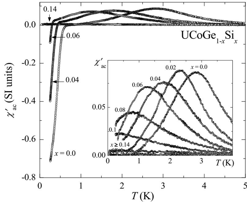
Figure 8.8 Temperature dependence of the ac-susceptibility of the  $\text{UCoGe}_{1-x}\text{Si}_x$  alloys for  $x = 0.0, 0.04, 0.06$  and  $0.14$ . The inset shows ac-susceptibility around the FM transition for  $x$  in the range  $0 \leq x \leq 0.2$ .
