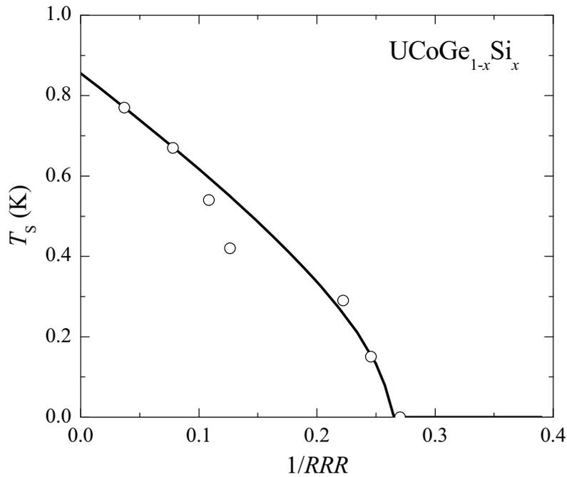
Figure 8.10 The superconducting transition temperature  $T_S$  as a function of  $1/RRR$  of the  $UCoGe_{1-x}Si_x$  alloys. The solid line is a fit of the data to the Abrikosov-Gor'kov pair-breaking function shown in Eq. 8.1 (for details see text).
