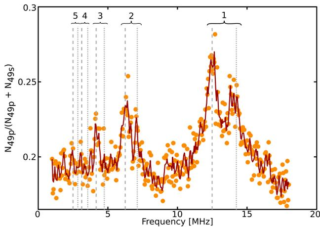
FIG. 7. (Color online) Observed frequency dependence of rf-assisted dipole-dipole transitions at  $F_S=0.26$  V/cm. Multiphoton peaks with  $n=1-5$  involved photons are clearly distinguishable; the number of involved photons is denoted in the figure. The double peak structure corresponds to the two resonances  $F_a$  and  $F_b$ . The solid line is a smooth spline fitted to the data.
