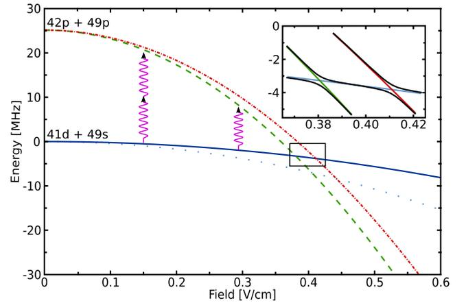
FIG. 3. (Color online) Schematic representation of two-atom energy versus electric field. An external rf field of 10 MHz is symbolized by the arrows. At a purely static field of 0.38 V/cm and 0.41 V/cm the dipole-dipole transition is resonant. At 0.3 V/cm it is brought into resonance by one rf photon of 10 MHz, while at 0.15 V/cm two such photons bring the system into resonance. The inset shows the avoided crossings due to dipole-dipole interaction at a separation of  $25 \mu\text{m}$ .
