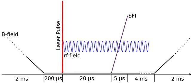
FIG. 4. (Color online) Schematic of the timing of one experimental cycle. First, the magnetic field is switched off, a laser pulse excites Rydberg states, which then are field ionized after 20- $\mu$ s interaction time. Finally, the magnetic field is switched on again.
