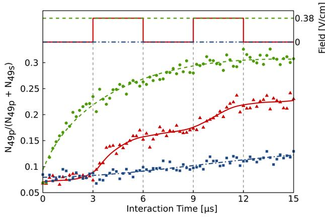
FIG. 6. (Color online)  $49p$  fraction as a function of interaction time for different fields  $F=F_a$  (green circles),  $F=0$  (blue squares), and  $F$  alternating between  $F_a$  and  $0$  in the manner depicted on top of the figure (red triangles). Lines depict a smooth spline fitted to the data.
