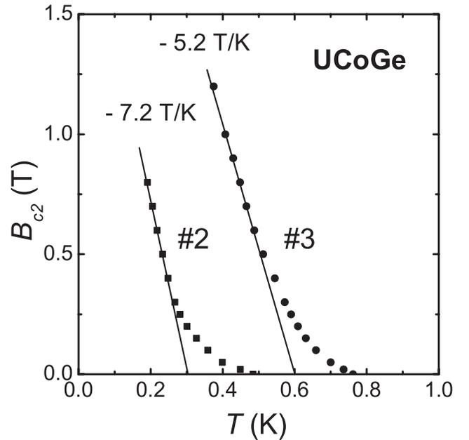
FIG. 4. Upper critical field  $B_{c2}$  determined by the midpoints of the resistive transitions measured in fixed magnetic fields. The solid lines indicate  $B_{c2}/dT = -7.2$  and  $-5.2$  T/K for samples 2 and 3, respectively, and extrapolate to zero field  $T_s$  values of 0.30 and 0.60 K.
