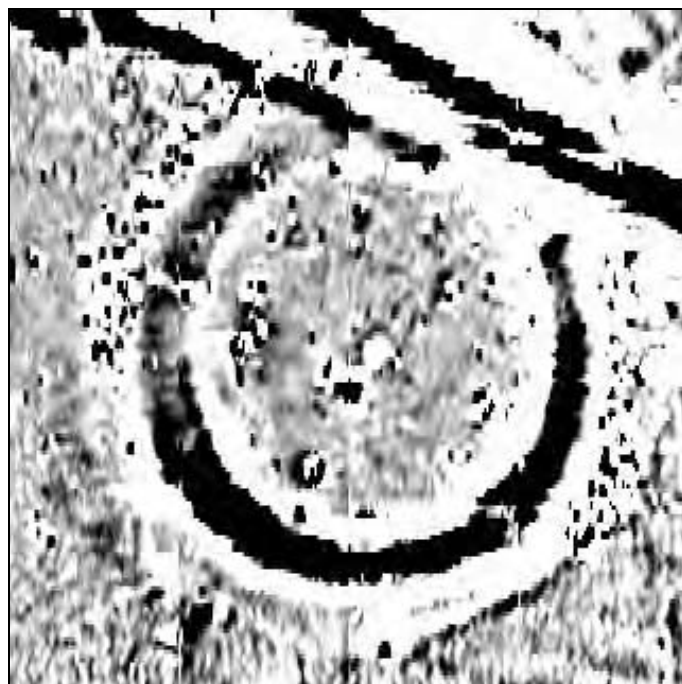
Figure 1 Magnetometer dataplot of the survey that was conducted by GSB Prospection at the Neolithic site the Standing Stones of Stenness, Orkney, United Kingdom. This is not the original dataset but the result of a repeated survey 25 years later. Extend 80 x 80 meter, range 0 (white) to 20 nT (black). Figure has been reproduced with kind permission.
