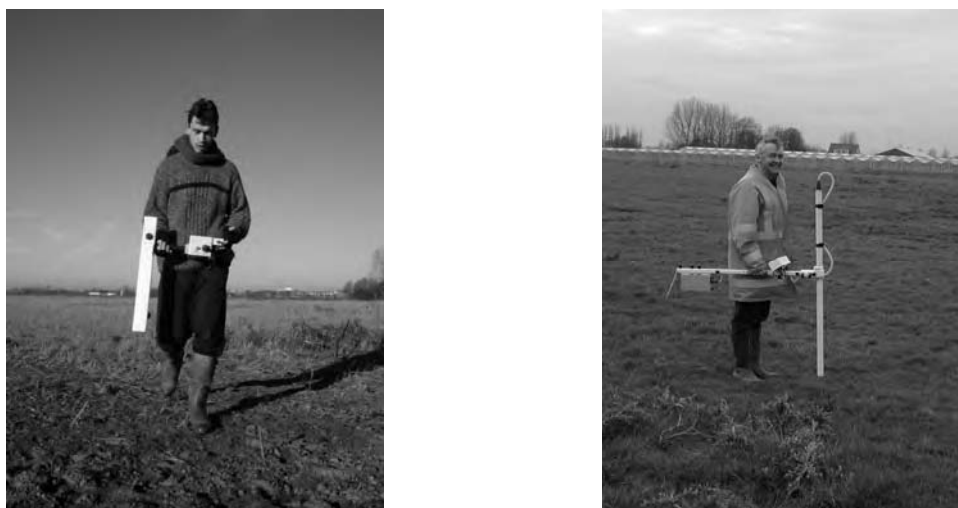
Figure 13 A Geoscan fluxgate gradiometer with 0.5 meter sensor separation (left) and a Bartington fluxgate gradiometer with 1 meter sensor separation (right).
