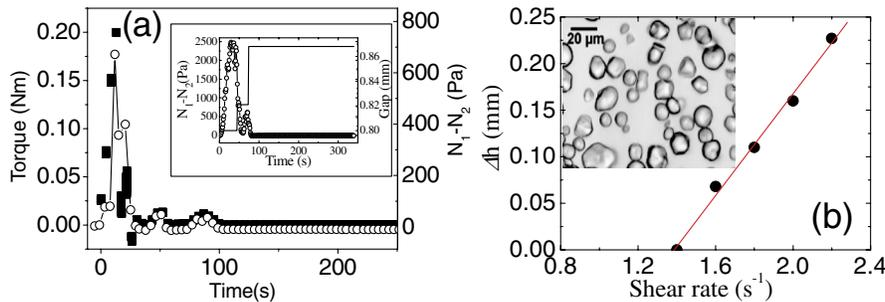
FIG. 4 (color online). (a) Time evolution of the torque and the normal stress for  $\dot{\gamma} = 1.6 \text{ s}^{-1}$ . Inset: Evolution of the normal stress and the gap. Torque (squares),  $N_1 - N_2$  (circles), gap (line). (b) Variation of the gap according to the shear rate. Inset: Micrograph of the cornstarch particles.
