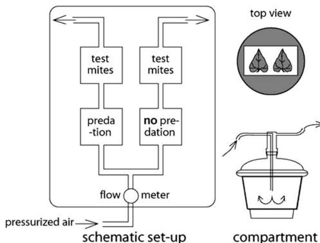
**Fig. 1** Exposure of spider mites to volatile predator-associated cues in a setup with two parallel sets of serial compartments. Arrows indicate a unidirectional continuous air stream. Odour sources were placed in the upwind compartments, odour-exposed leaves in the downwind compartments (*test mites*). An odour source consisted of two bean leaves either infested with spider mites and predatory mites (*predation*), or with spider mites alone (*no predation*)
