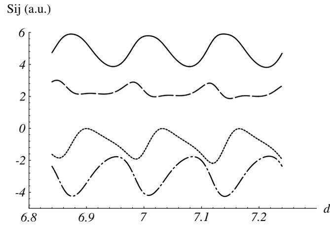
Figure 7: The integrated scattering matrix elements, as a function of the diameter  $d$  of the sphere;  $d$  is in micrometer, the  $s_{ij}$  are in arbitrary units; the solid line is  $s_{11}$ ; the dotted line is  $s_{12}$ ; the dashed line is  $s_{33}$ ; the dashed-dotted line is  $s_{34}$ .
