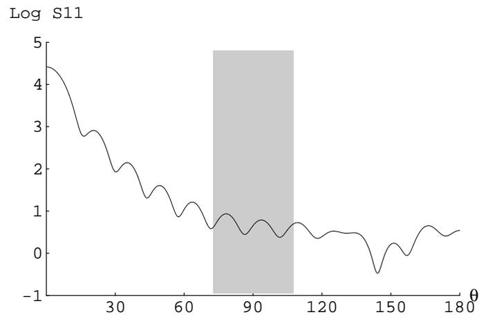
Figure 8: The  $S_{11}$  element as a function of the scattering angle  $\theta$ , for  $d = 1.98 \mu\text{m}$ . The grey area denotes the field of view of the side scattering detectors.
