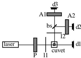
Figure 1: Schematic drawing of the optical system of the FlowCytometer. The laser beam is focussed by lens **l1** on a cell, flowing through the cuvet. The incident beam is polarized by means of the polarizer **P**. The intensity of the forward scattered light is measured by detector **d1**, the sideward scattered light is focussed by lens **l2** on detectors **d2** and **d3**, **bs** is a beamsplitter. The side scattering signals are passed through two different analyzers **A1** and **A2**.
