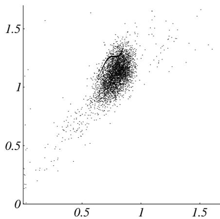
Figure 6: The normalized experimental and theoretical  $(s_{11}+s_{12}, s_{11}-s_{12})$  scatterplot for polystyrene spheres with a mean diameter of  $1.98 \mu\text{m}$ . The horizontal axes is the  $s_{11}+s_{12}$  signal in the sideward direction, the vertical axes is the  $s_{11}-s_{12}$  signal in the sideward direction.
