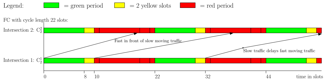
Figure 8.3: Illustration that green waves under coordinated FC are lost when car speeds vary: the I2F4C2 case with \rho_1 = \rho_2 = 0.8 and ideal distance T_{1,2} = 22 slots (=611 meters).
