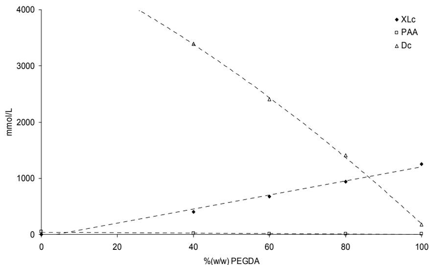
Fig. 2.14. Various parameters of the network for the different UV-cured PEGDA/EHA networks.
