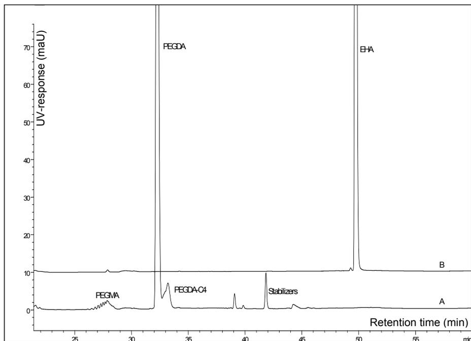
Fig. 2.2. UV-chromatogram ( $\lambda = 210$  nm) of PEGDA (A) and EHA (B). Conditions: 250 $\times$ 3 mm ODS-3, 0.5 mL/min, 40°C, 5  $\mu$ L, gradient; 0–5 min, 100% H<sub>2</sub>O, 5–45 min from 0–100% acetonitrile, where it remains constant for 15 min.
