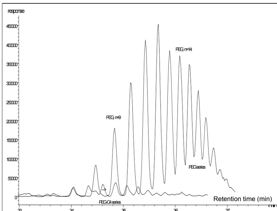
Fig. 2.6. Mass-reconstructed chromatogram of PEG and PEG- $C_4$  of a hydrolysed PEGDA/EHA(60:40) sample analysed by SEC-LC. Conditions;  $8 \times 300$  mm Suprema 1000  $\text{\AA}$  coupled to  $250 \times 4.6$  mm ODS-3 column, 1.0 mL/min, 20  $\mu\text{L}$ , RT, gradient; 0–10 min, 100% 0.1 M  $\text{NH}_4\text{Ac}$ , 10–30 min from 0–50% acetonitrile, where it remains constant for 30 min.
