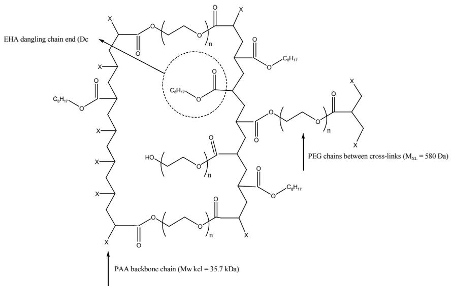
Fig. 2.11b. Chemical network structures of PEGDA/EHA (60:40).
