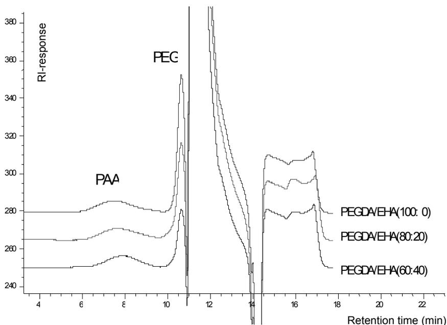
Fig. 2.3. SEC-chromatograms of hydrolysed UV-cured PEGDA/EHA polymers using RI-detection;  $8 \times 300$  mm Suprema column (PSS),  $1000 \text{ \AA}$ ,  $10 \text{ \mu m}$ , flow =  $1.0 \text{ mL/min}$   $0.1 \text{ M NH}_4\text{Ac}$ ,  $T = 25^\circ\text{C}$ ,  $V_{inj} = 20 \text{ \mu L}$ .
