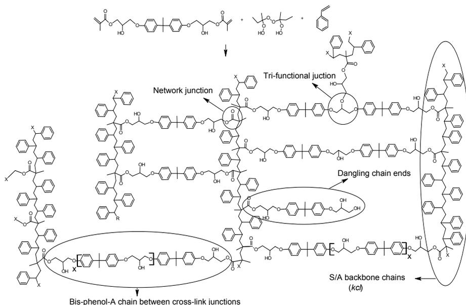
Fig. 3.13. Styrene/di-methacrylate network structure as determined by different analysis techniques.
