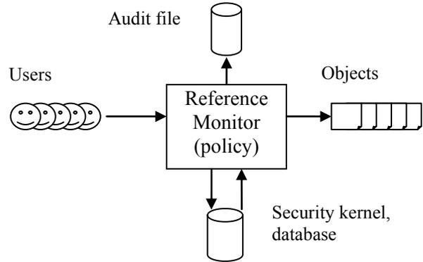
Figure 3. Reference Monitor model (applied in an “orthogonal” way to all system calls).
