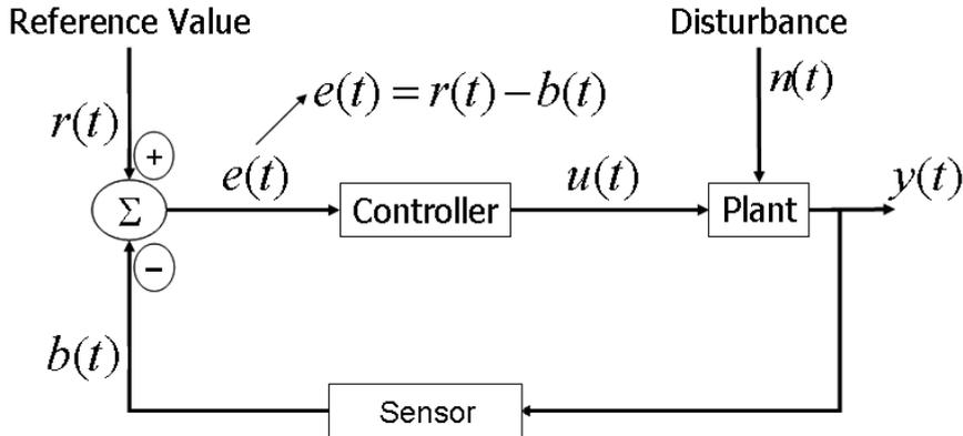
**Figure 1.5. Elementary control system.**  $y(t)$  : the plant output and measured signal;  $u(t)$  : the plant input (i.e., actuating signal);  $n(t)$  : the external disturbance;  $b(t)$  : sensor output;  $r(t)$  : reference or command input;  $e(t)$  : error or deviation (this figure is based on Ref. 61).
