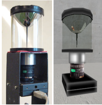
Figure 1: The catadioptric omnidirectional camera, real and simulated.
