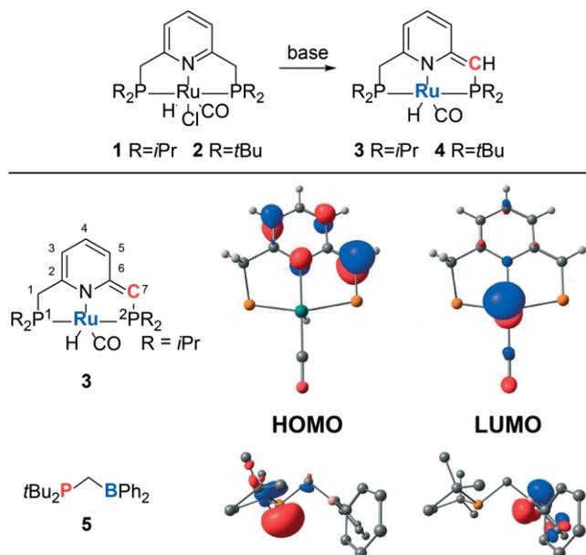
Figure 1. Top: Milstein system, activation of precursor by deprotonation with a base resulting in the dearomatized species. Bottom: molecular orbital diagram of MLC **3** (isopropyl groups omitted for clarity) and FLP **5** (left: HOMO, right: LUMO) calculated at the  $\omega\text{B97X-D}/6\text{-311G(d,p)}$  level of theory. Blue: Lewis acid; red: Lewis base.
