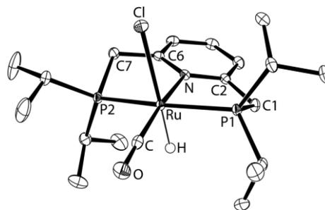
Figure 8. Molecular structure of **1** [(*i*PrPNP)RuHCl(CO)] (displacement ellipsoids are set at 50 % probability, hydrogen atoms omitted for clarity). Selected bond lengths [Å]: Ru–P1 2.3221(4), Ru–P2 2.3061(4), P1–C1 1.8415(14), P2–C7 1.8435(15), C1–C2 1.5051(19), C6–C7 1.501(2).
