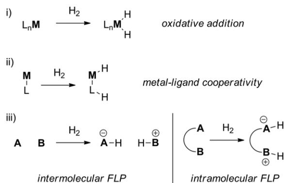
Scheme 1. Differing modes of dihydrogen activation by transition metal complexes and frustrated Lewis pairs (**M** = transition metal, **A** = Lewis acidic site, **B** = Lewis basic site, **L** = ligand).
