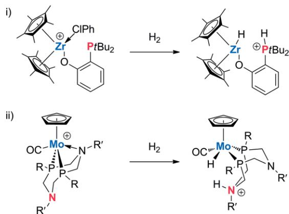
Scheme 2. Transition metal-based FLP reactivity, and/or MLC reactivity: activation of dihydrogen by i) Wass's Zr complex<sup>[8]</sup> and ii) Bullock's Mo complex.<sup>[11]</sup> Blue: Lewis acid; red: Lewis base.
