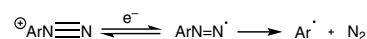
Scheme 14 Arenediazonium salt undergoing one-electron reduction, formation of the intermediate diazenyl radical before losing \text{N}_2 (counter-ion omitted)
