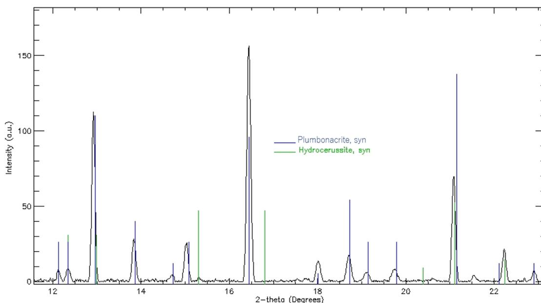
Figure S.3 : Diffractogram collected on a droplet of cured oil (heated without any Pb source) with dispersed PbO particles, left to dry for 3 months at 60°C.
