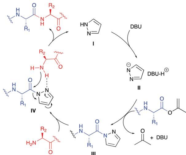
**Scheme 2** Proposed catalytic cycle for the pyrazole catalysed aminolysis of isoprenyl esters.
