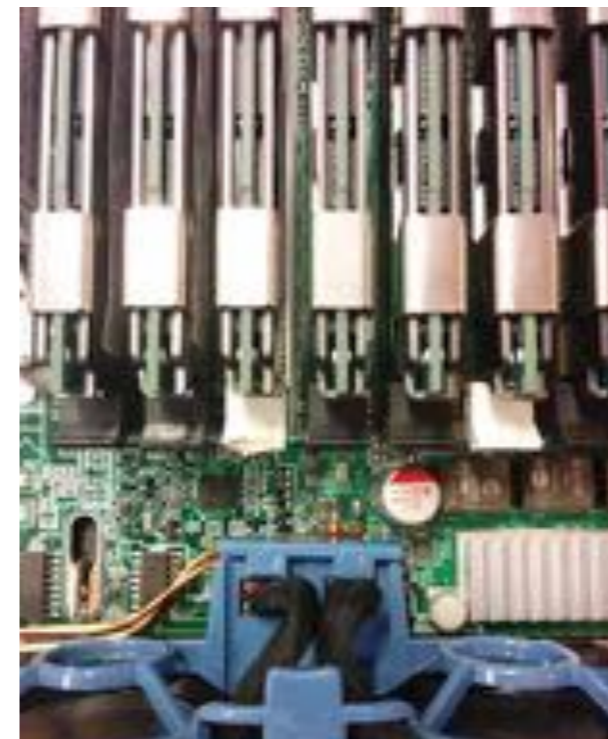
Figure 3.1 Wires soldered on motherboard to measure energy consumption of memory.
