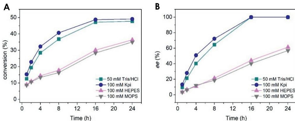
**Figure 2.** KR of *rac*-**1a** (10 mM) catalyzed by LE-AmdH-v1 (45  $\mu$ M) and using different types of buffers with NAD<sup>+</sup> (1 mM) and NO<sub>x</sub> (3  $\mu$ M) at 30 °C. (A) Progress of the KR over the time. (B) Variation of the ee of the unreacted enantiomer over the time.
