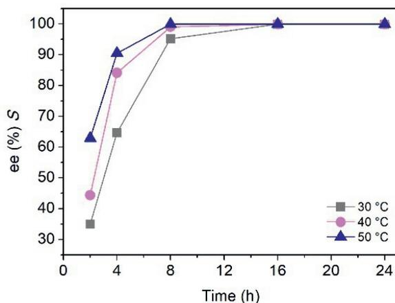
Figure 3. Progress of the KR of *rac*-1a (10 mM) at different temperatures (30 °C- 50 °C) catalyzed by LE-AmDH-v1 (90 μM) with NAD<sup>+</sup> (1 mM) and NO<sub>x</sub> (10 μM).
