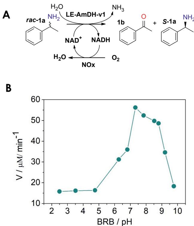
**Figure 1.** (A) Schematic representation of the reactions performed. (B) Reaction rate of the oxidative deamination of *rac*-1a at different pH values using Britton–Robinson's universal buffer. Catalytic amount of NAD<sup>+</sup> (1 mM) was applied and recycled using the NO<sub>x</sub> (3 μM). All reactions (0.5 mL) were performed at 40 °C using 10 mM of **1a** and 45 μM of LE-AmDH-v1. Reaction times varied from 5 to 40 min.
