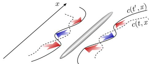
FIG. 1. Prototypical experimental setup that can be addressed with our method. A Bose gas is trapped in a one-dimensional tube. The space-time dependent interparticle interaction strength  $c(t, x)$  is modified by modulating the transverse trapping potential (see also Fig. 2).
