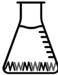
Figure S2. Schematic depiction of SR sheets stacked in harmonica shape at the bottom of an Erlenmeyer flask for the extraction of the organic compounds.
